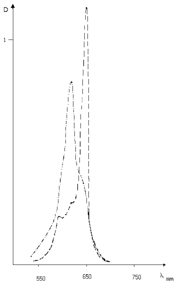
Fig. 1. The electronic adsorption spectra \text{Zn}(4\text{-SO}_3\text{Na})_4\text{Pc} in (—) water solutions (---) water-alkaline medium after ethanol addition (0.3:1, v/v).
