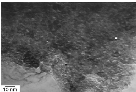
Fig. 3. HREM micrograph of Zr_{0.70}Y_{0.10}Er_{0.05}Ce_{0.15}O_{1.925} gel powder decomposed at 700 °C for 30 min.
