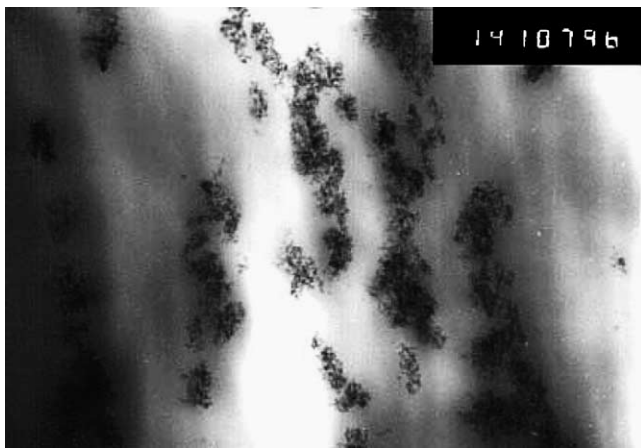
Fig. 2. TEM microphotograph of PP/surface-treated SiO 2 containing 10 wt.% silica nanoparticles.
