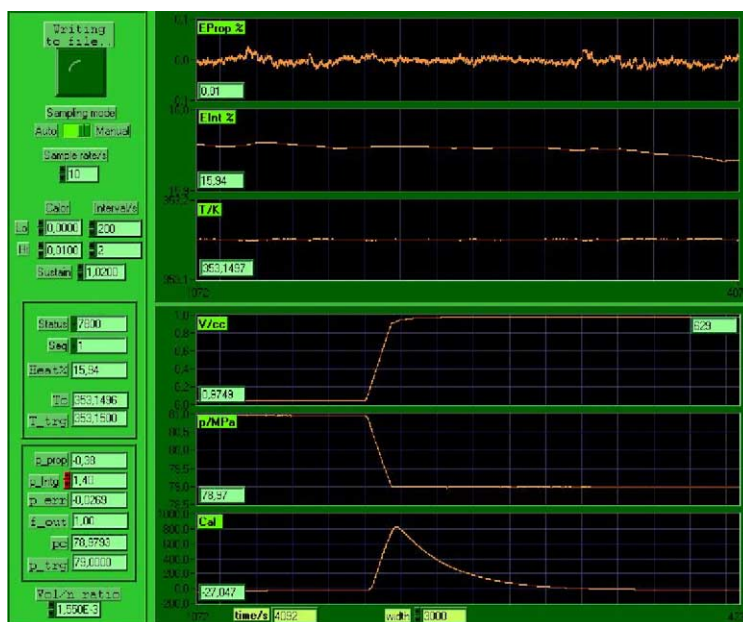
Fig. 2. A window with a typical general view of the LabView software output (pressure decrease under isothermal conditions).
