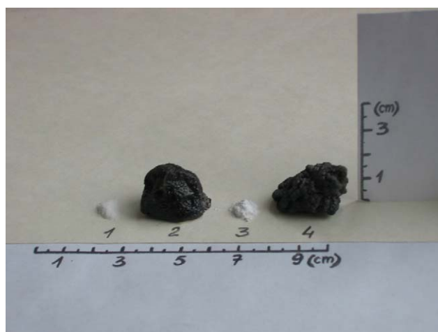
Fig. 3. PEPA (50 mg) before (1) and after (2) exposure to flame. PEPAMP (50 mg) before (3) and after (4) exposure to flame.
