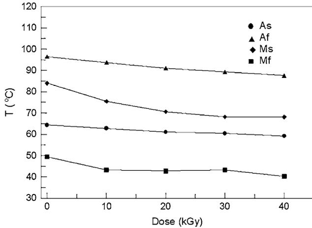
Fig. 2. Changes of transformation temperatures with the dose of gamma irradiation in CuZnAl alloy.
