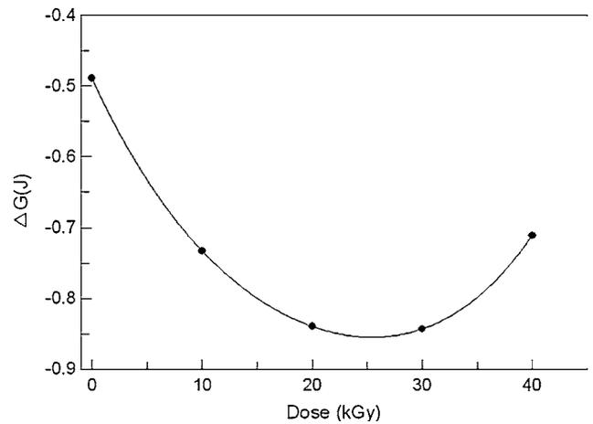
Fig. 4. Changes of Gibbs free energy with the dose of gamma irradiation in CuZnAl alloy.
