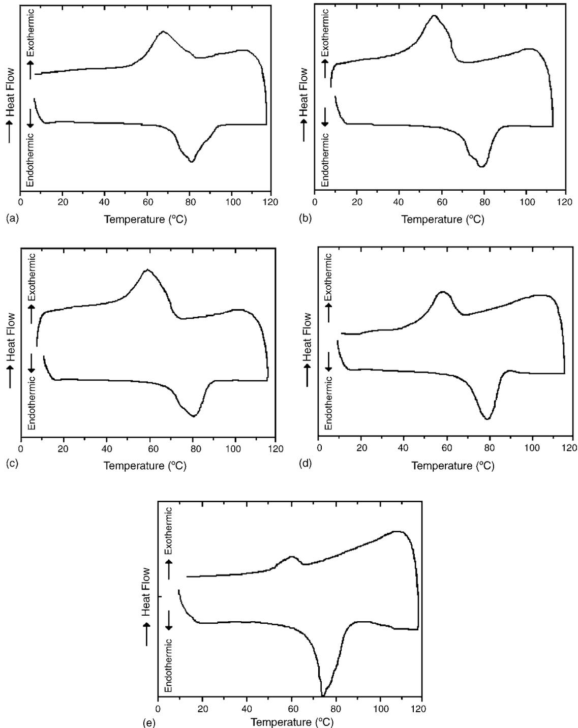
Fig. 1. DSC curves of the alloy at various doses (a) unirradiated (b) 10 kGy (c) 20 kGy (d) 30 kGy (e) 40 kGy.
