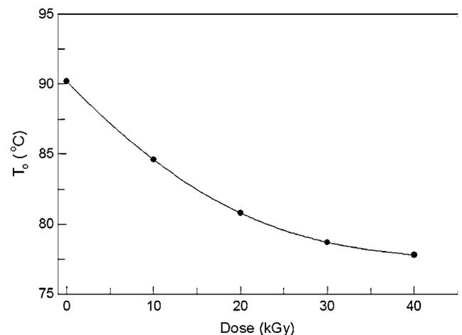
Fig. 5. Effect of gamma irradiation on the equilibrium temperature of the alloy.
