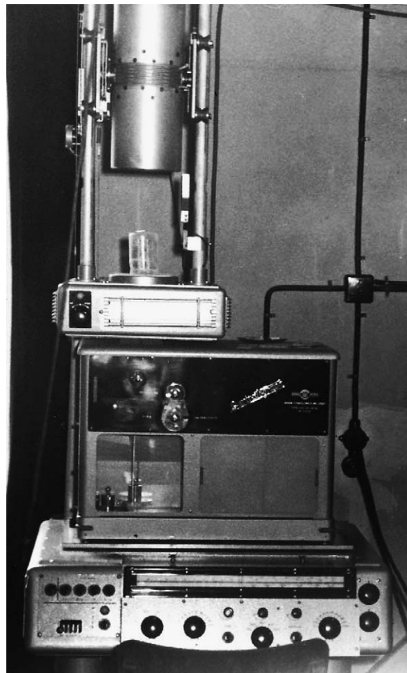
Fig. 1. Derivatograph, built 1964, at the former Mineralogical Institute of the Friedrich-Schiller University in Jena, Germany.
