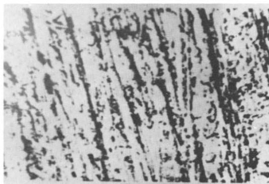
Fig. 1. Microstructure of the \alpha -naphthol-catechol eutectic [6]. \times 50 .
