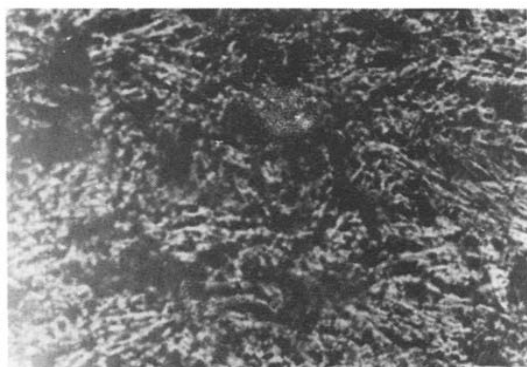
Fig. 3. Microstructure of the \beta -naphthol-catechol eutectic containing \alpha -naphthol impurity. \times 50 .
