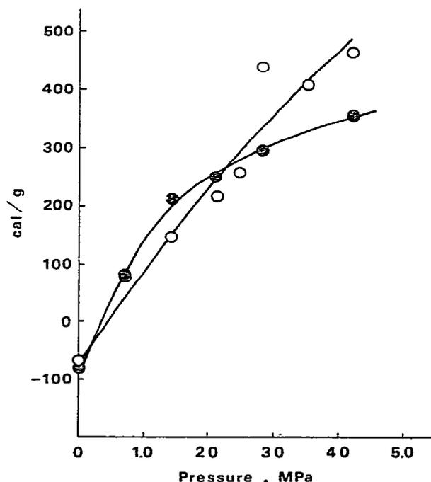
Fig. 3. Variation of decomposition heats of CT in nitrogen or air with pressure. Heating rate:  $10^{\circ}\text{C min}^{-1}$ . ○,  $\text{N}_2$ ; ●, air.
