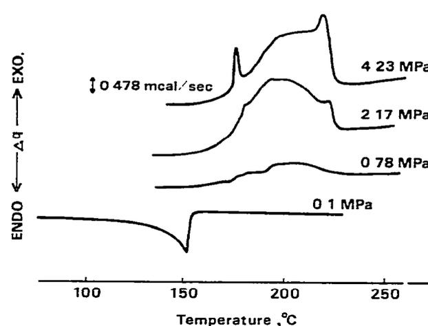
Fig. 1. DSC curves of CT in nitrogen at various pressures. Heating rate:  $10^{\circ}\text{C min}^{-1}$ .
