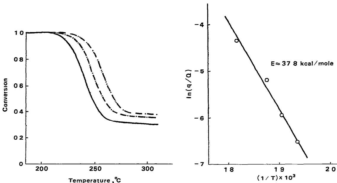
Fig. 14. TG curves of AAT in helium at 2.06 MPa at various heating rates. Weight  $\sim 5$  mg. —,  $2.5^\circ\text{C min}^{-1}$ , - - - - ,  $5^\circ\text{C min}^{-1}$ ; - · - · -,  $10^\circ\text{C min}^{-1}$ .
