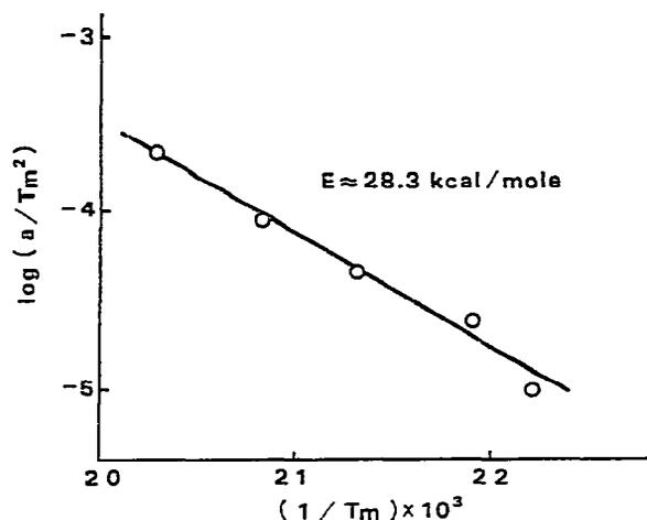
Fig. 8. Kissinger's plots of CT in nitrogen at 4.23 MPa.
