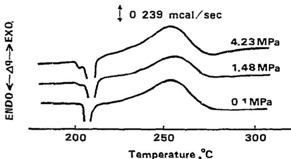
Fig. 13. DSC curves of AAT in nitrogen at various pressures. Heating rate:  $10^\circ\text{C min}^{-1}$ .
