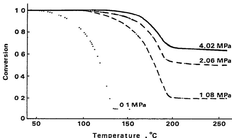
Fig. 6. TG curves of CT in helium at various pressures. Heating rate  $10^{\circ}\text{C min}^{-1}$ , weight  $\sim 5$  mg.
