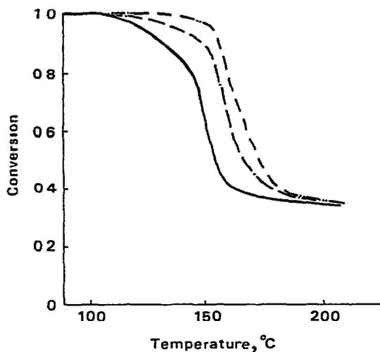
Fig. 11. TG curves of AT in helium at 2.06 MPa at various heating rates. Weight  $\sim 5$  mg. —,  $2.5^\circ\text{C min}^{-1}$ ; - - -,  $5^\circ\text{C min}^{-1}$ ; - · - ·,  $10^\circ\text{C min}^{-1}$ .
