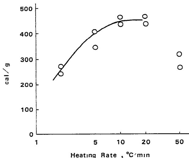
Fig. 4. Influence of heating rates on decomposition heats of CT in nitrogen at 4.23 MPa.
