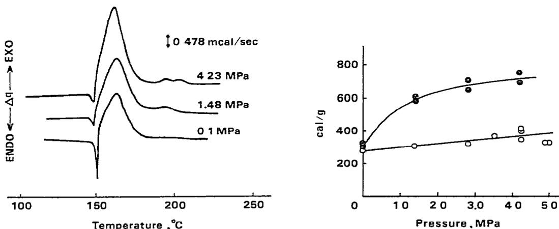
Fig. 9. DSC curves of AT in air at various pressures. Heating rate:  $10^\circ\text{C min}^{-1}$ .
