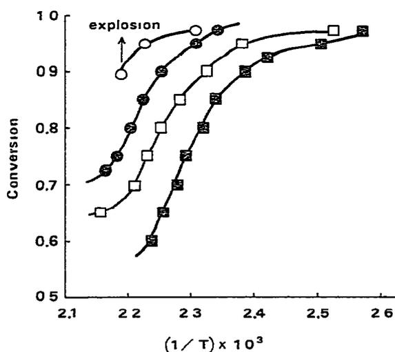
Fig. 7. Variation of TG curves of CT in helium at  $4.02 \text{ MPa}$  with various heating rates, plotted against the reciprocal of absolute temperature. Weight:  $\sim 10$  mg.  $\circ$ ,  $10^{\circ}\text{C min}^{-1}$ ,  $\bullet$ ,  $5^{\circ}\text{C min}^{-1}$ ;  $\square$ ,  $2.5^{\circ}\text{C min}^{-1}$ ,  $\blacksquare$ ,  $1.25^{\circ}\text{C min}^{-1}$ .
