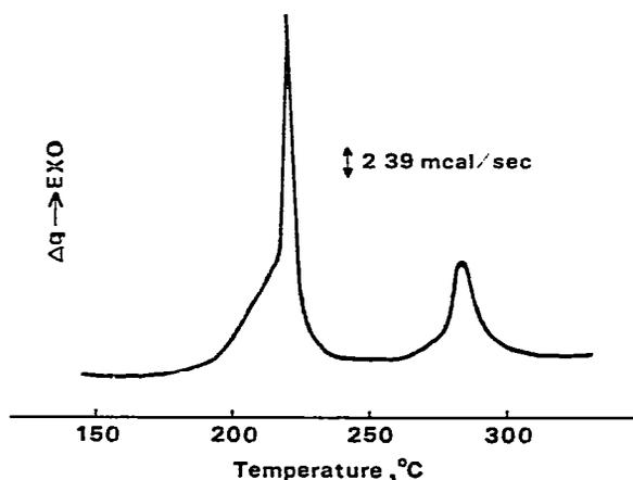
Fig. 5. Pressure DSC curve of CT in nitrogen at 4.23 MPa. Heating rate:  $50^{\circ}\text{C min}^{-1}$ .
