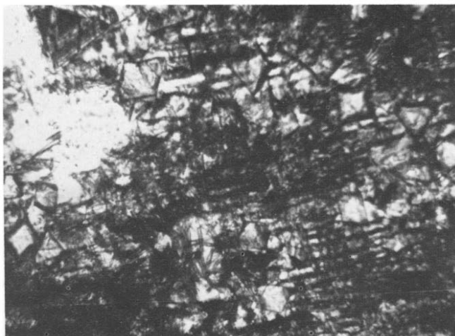
Fig. 9. Photomicrograph of G9-5.0% \text{TiO}_2 + 0.2% \text{ZrO}_2 ; slow cooling regime. Growths of \beta -spodumene ss crystals with fine gahnite octahedrons, diopside microlites, and needles of rutile. Crossed nicols, \times 250 .
