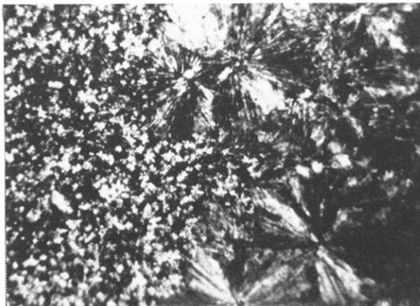
Fig. 5. Photomicrograph of G9-2.5% TiO 2 ; 780°C/2 h. Minute star-like skeletal and radial fibrillar growths of \beta -eucryptite ss and pyroxene exhibiting heterogeneous coarse-grained texture. Crossed nicols, \times 62 .
