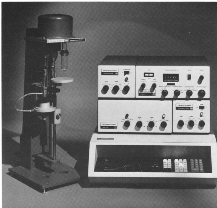
Fig. 1. Perkin-Elmer TGS-2 thermogravimetric analysis system with system 4 microcomputer controller.
