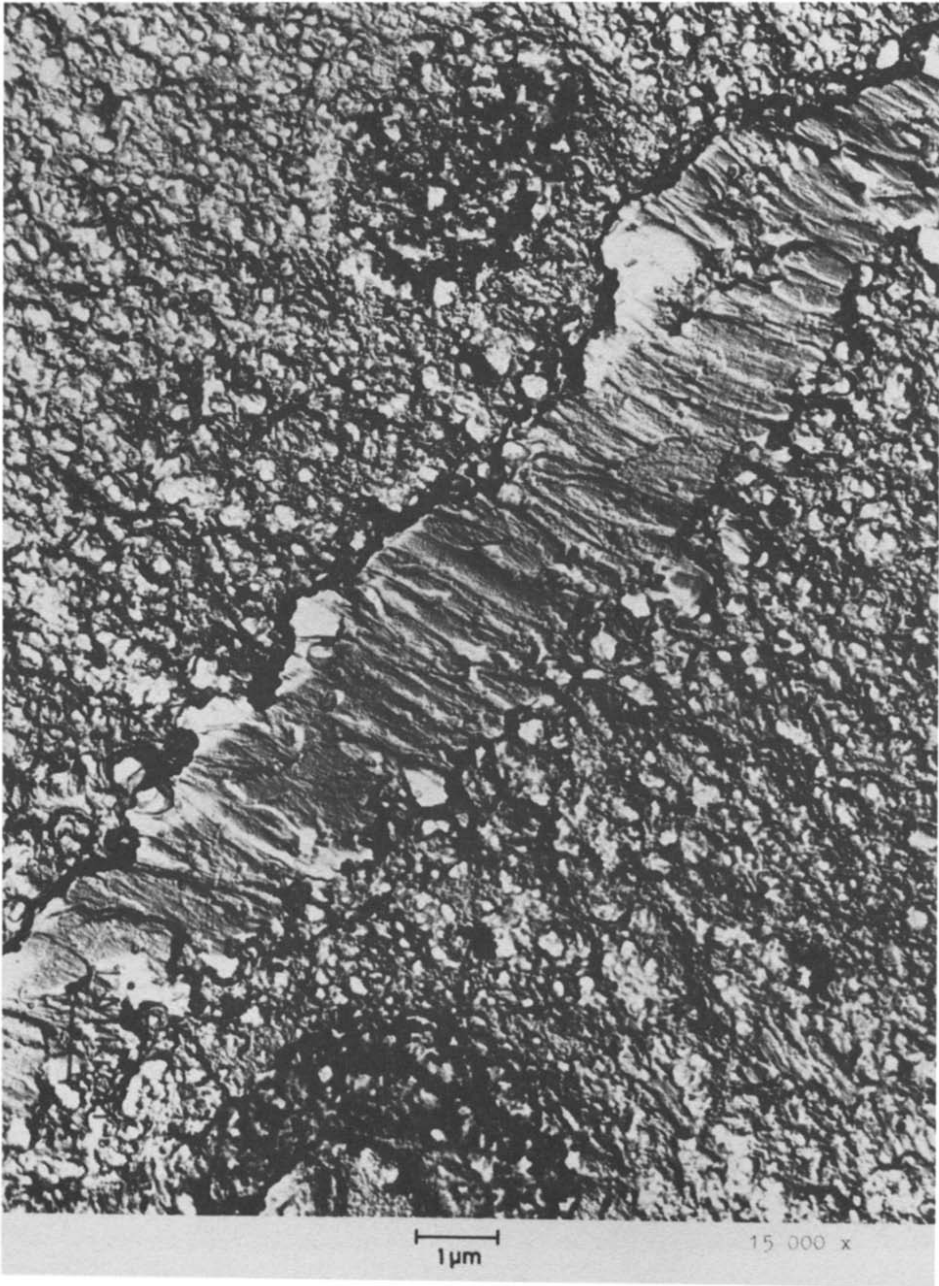
Fig. 4. PbNa cast alloy with the grain boundary filled with a separate phase of NaPb-Na 2 Pb 5 eutectic.
