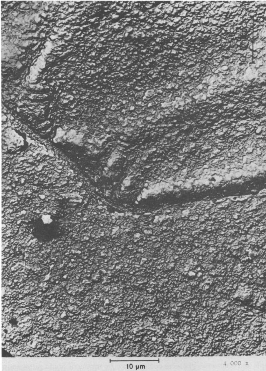
Fig. 3. PbNa flake alloy with grain boundary.
