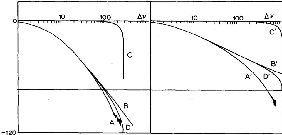
Fig. 1. Experimental transfer function (modulus in dB and phase in rad) of the JLM-E1 conduction calorimeter (A and A'). B and B' are the analytic approximations to the TF; C and C' are the frequential representations of the integral smoothing over  $T_c$ ; D and D' are the analytical models plus the corresponding filter. (Unprimed capital letters stand for dissipations far from the detector system whereas primed ones correspond to dissipations near the detectors).  $\Delta\nu = 1/2048$  Hz.
