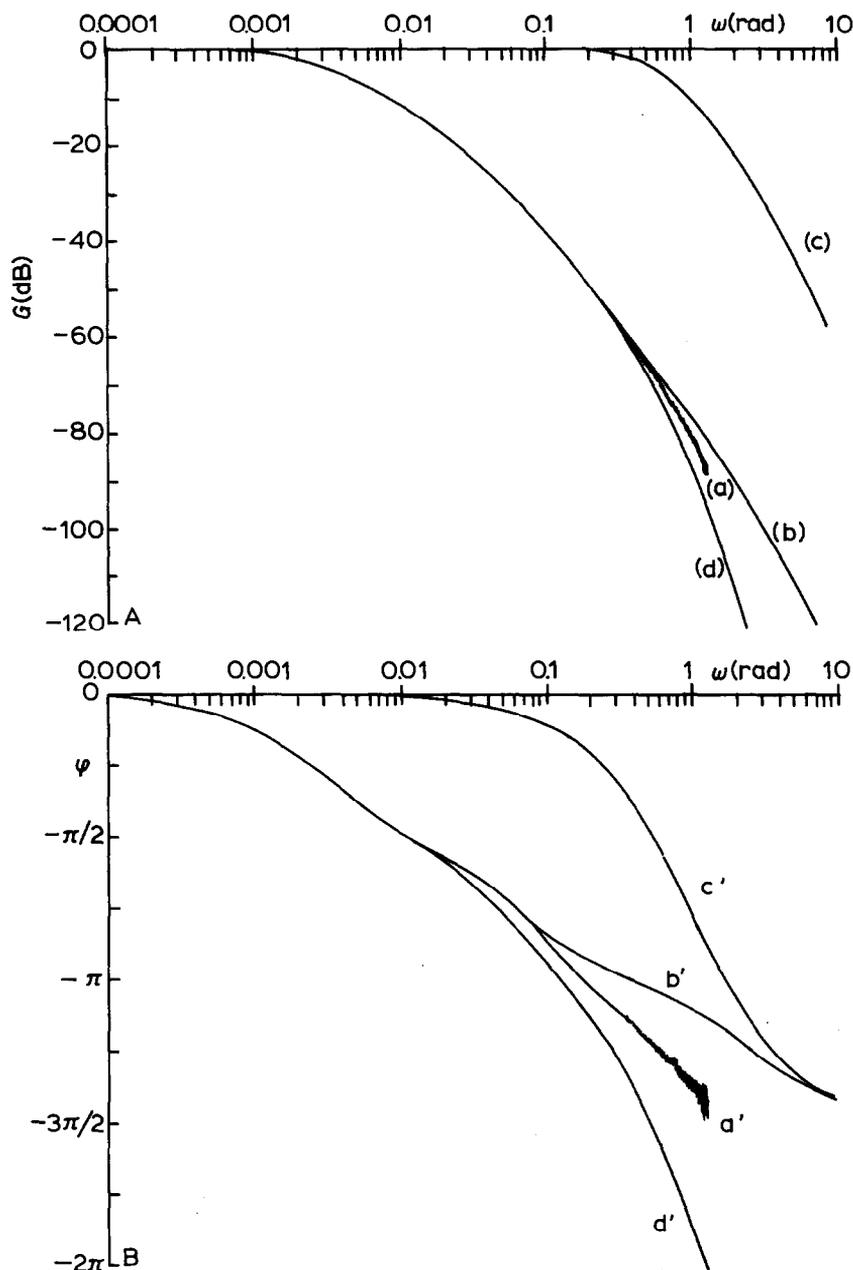
Fig. 2. Modulus (A) in dB and phase (B) in rad of: (a) experimental TF of STQ. ADA calorimeter; (b) model ( $\tau_1 = 378.0$  s,  $\tau_2 = 17.0$  s,  $\tau_3 = 0.4$  s); (c) compensating plant (three poles  $\tau^* = 1.02$ ); (d) model plus compensating plant.
