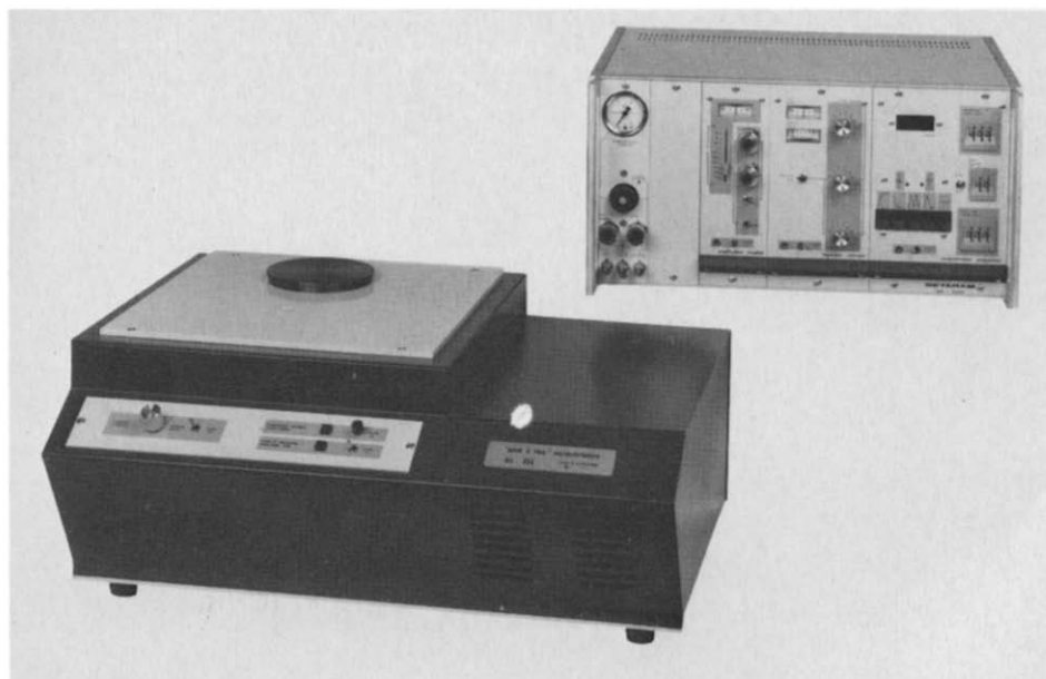
Figure 1 - Photograph showing the BIO-DSC "Batch and Flow" calorimeter.
