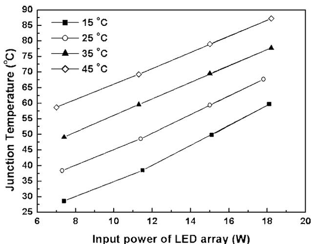
Fig. 7. Junction temperature of LED array with heat pipe at dipping liquid temperature of  $15^\circ\text{C}$ ,  $25^\circ\text{C}$ ,  $35^\circ\text{C}$ ,  $45^\circ\text{C}$ .
