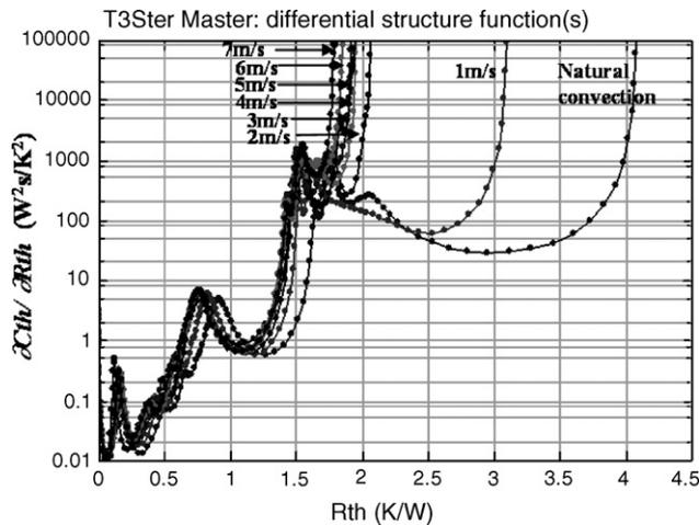
Fig. 6. Differential structure functions from the LED array with heat pipes.
