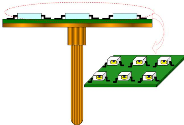
Fig. 1. Schematic structure of an LED array mounted on MCPCB.
