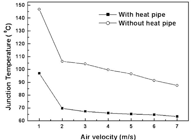
Fig. 5. Comparison of junction temperature of LED array without and with heat pipes under different air velocity.
