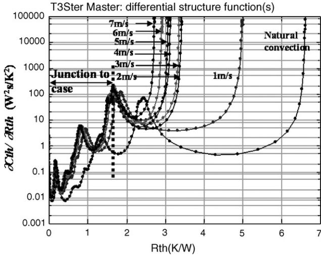
Fig. 3. Differential structure functions of LED array as a function of convection condition (without heat pipes).
