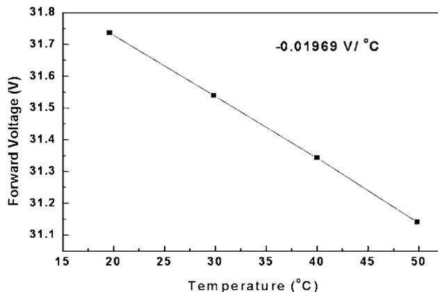
Fig. 2. Forward voltage vs. temperature plot showing a  $K$  factor of LED array.
