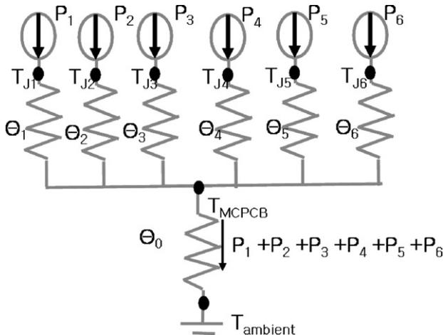
Fig. 4. Equivalent circuit of LED arrays investigated in this study.
