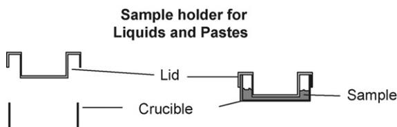
Fig. 1. Sample holder system for liquids and pastes for flash instruments.
