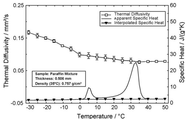
Fig. 6. Apparent thermal diffusivity and apparent specific heat of a paraffin mixture.
