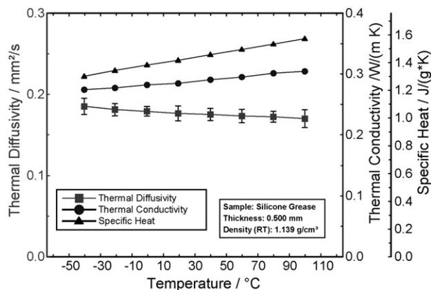
Fig. 5. Thermal diffusivity, specific heat and thermal conductivity of a silicon grease.
