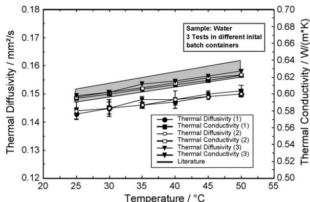
Fig. 2. Thermal diffusivity and thermal conductivity of water measured with the new sample holder for liquids and pastes.
