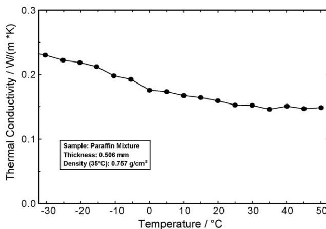
Fig. 7. Thermal conductivity of the paraffin mixture between  $-30$  and  $50$  °C.
