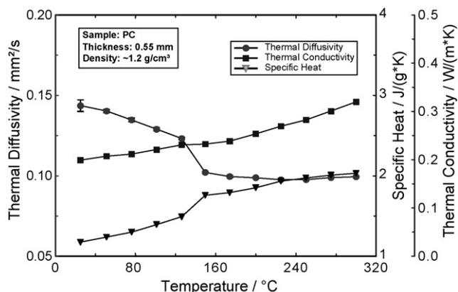
Fig. 4. Thermal diffusivity, specific heat and thermal conductivity of polycarbonate (PC).
