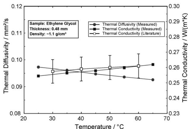
Fig. 3. Thermal diffusivity and thermal conductivity of ethylene glycol measured with the new sample holder for liquids and pastes.
