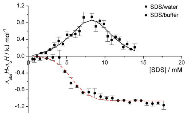
Fig. 4.  $(\Delta_{\text{obs}} H - \Delta_0 H)$  vs. SDS concentration for the dilution of SDS into water and SDS into buffer.
