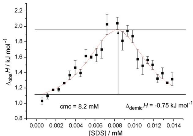
Fig. 2. Enthalpy per injection vs. concentration of SDS in the calorimetric ampoule for dilution of SDS into water.
