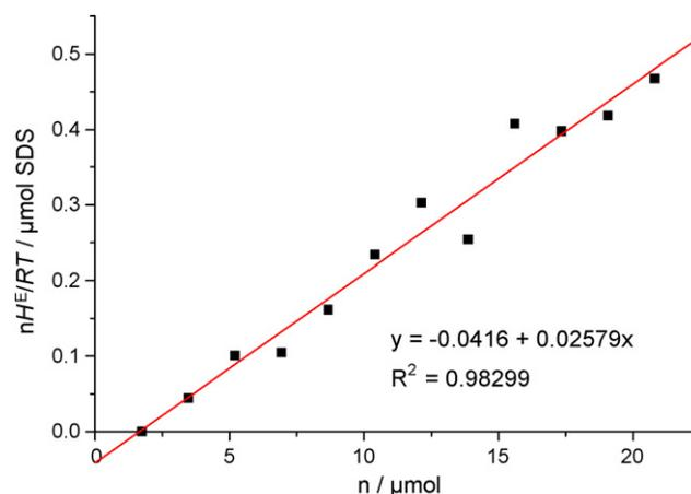
Fig. 5.  $nH^E/RT$  vs.  $n$  for the dilution of SDS into water.
