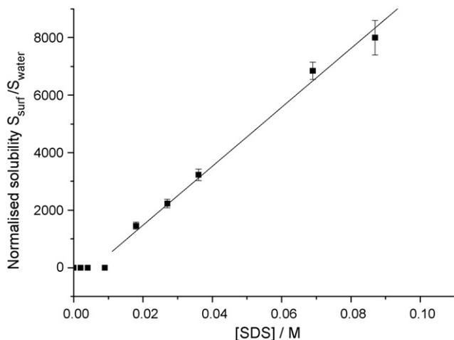
Fig. 1. Solubility enhancement curve for simvastatin in aqueous SDS solutions.
