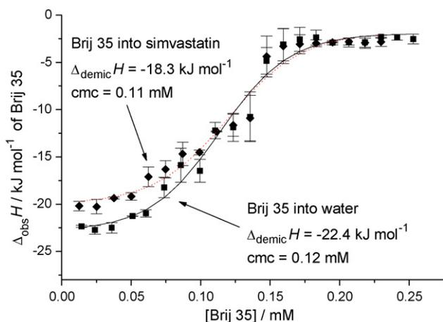
Fig. 9. Enthalpy per injection vs. concentration of Brij 35 in the calorimetric ampoule for dilution of Brij 35 into simvastatin solution and into water.
