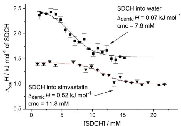
Fig. 8. Enthalpy per injection vs. concentration of SDCH in the calorimetric ampoule for dilution of SDCH into simvastatin solution and into water.
