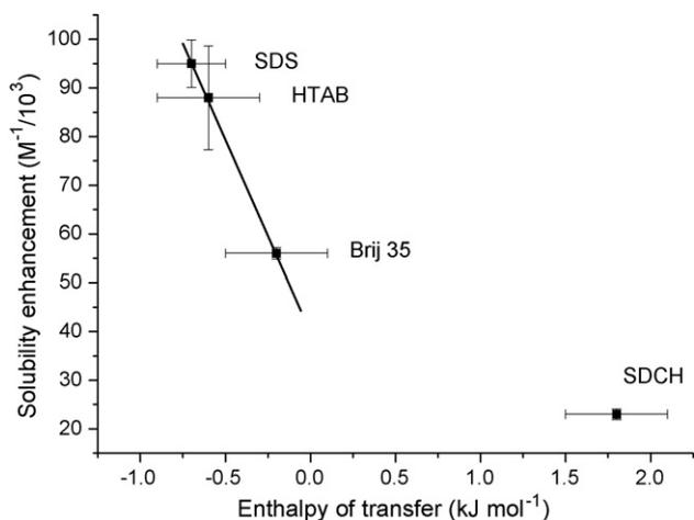
Fig. 10. A plot of the free energy of transfer of simvastatin into the surfactant micelles vs. the solubility enhancement; the data show a linear for those systems with a favourable free energy of transfer.
