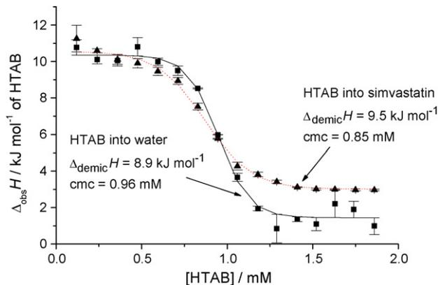
Fig. 7. Enthalpy per injection vs. concentration of HTAB in the calorimetric ampoule for dilution of HTAB into simvastatin solution and into water.
