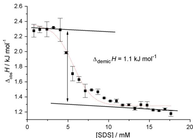
Fig. 3. Enthalpy per injection vs. concentration of SDS in the calorimetric ampoule for dilution of SDS into pH 7.0 phosphate buffer.
