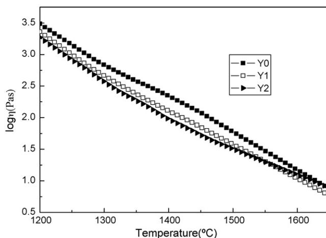
Fig. 1. Viscosity–temperature curves of Y0, Y1 and Y2.
