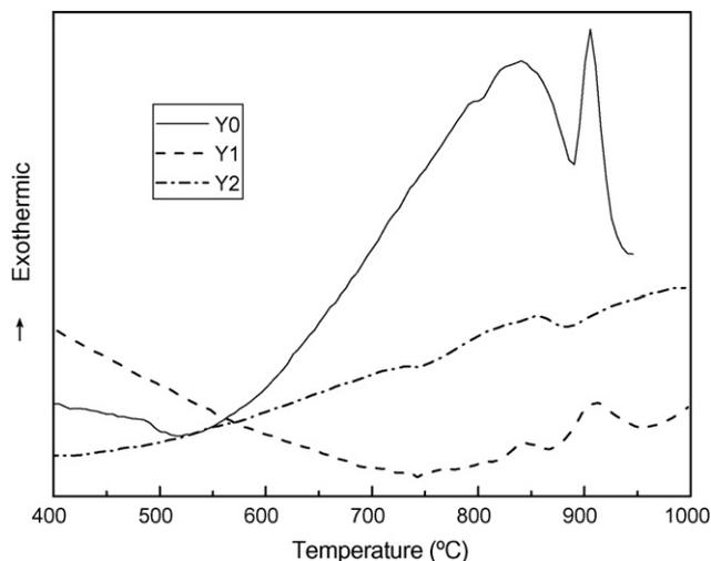
Fig. 2. DTA curves for glass samples with various  $Y_2O_3$  content at  $10^\circ C\ min^{-1}$ .
