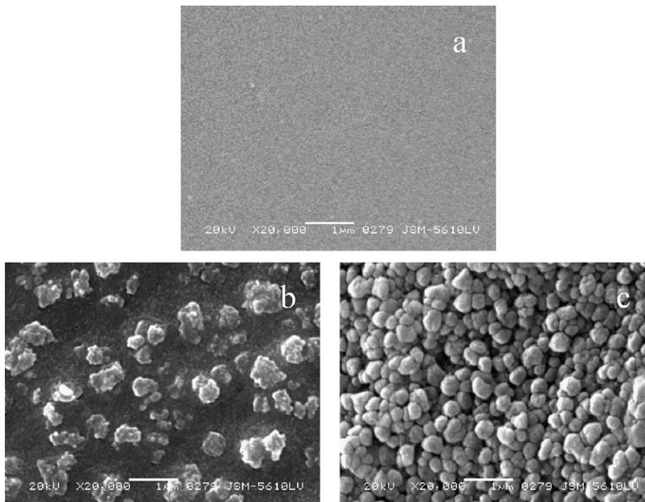
Fig. 5. SEM photos of Y1 specimen heat-treated for 2 h at different crystallization temperature: (a) 820 °C, (b) 842 °C and (c) 920 °C.
