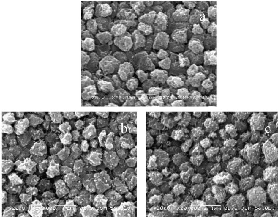
Fig. 4. SEM photos of Y0 specimen heat-treated for 2 h at different crystallization temperature: (a) 820 °C, (b) 870 °C and (c) 920 °C.
