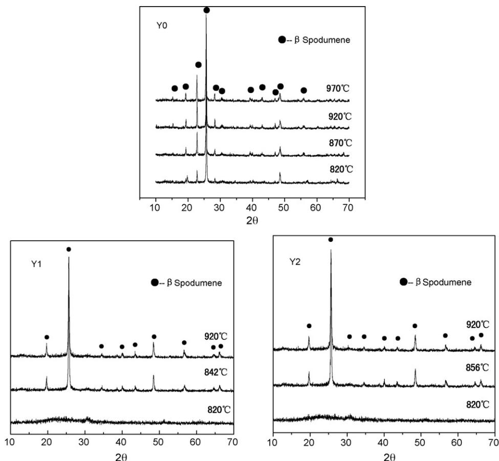
Fig. 3. XRD patterns of the three samples: Y0, Y1 and Y2.
