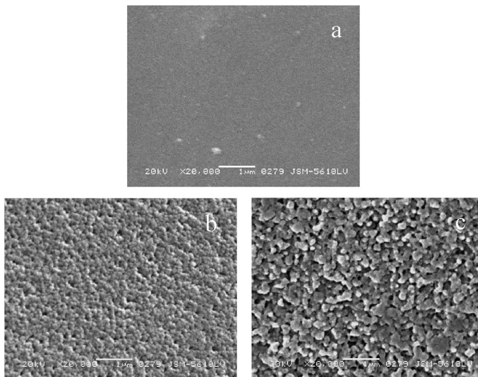
Fig. 6. SEM photos of Y2 specimen heat-treated for 2 h at different crystallization temperature: (a) 820 °C, (b) 856 °C and (c) 920 °C.
