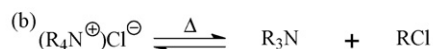
Scheme 1. Schematic representation of (a) Hoffmann elimination reaction; (b) SN_2 nucleophilic substitution reaction.
