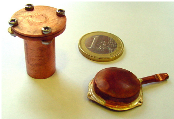
Fig. 1. Two main types of used calorimetric copper cells, compared to the size of an €1 coin.
