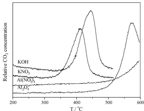
Fig. 1. TPR profiles (with soot coating) of individual compounds used for catalyst preparation.
