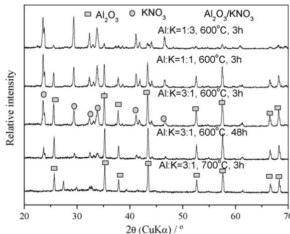
Fig. 6. XRD patterns of the catalysts prepared by  $\text{Al}_2\text{O}_3/\text{KNO}_3$  at various conditions.
