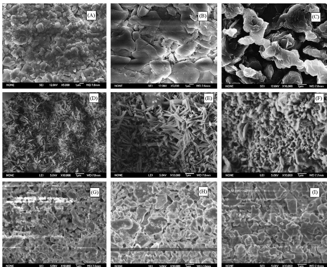
Fig. 7. Morphologies of the catalysts prepared with different precursors.  $\text{Al}_2\text{O}_3/\text{KOH}$  (Al:K = 1:1, (A) 600 °C, 3 h; (B) 700 °C, 3 h; (C) 600 °C, 48 h),  $\text{Al}(\text{NO}_3)_3/\text{KNO}_3$  (Al:K = 1:1, (D) 600 °C, 3 h; (E) 700 °C, 3 h; (F) 600 °C, 48 h) and  $\text{Al}_2\text{O}_3/\text{KNO}_3$  (Al:K = 3:1, (G) 600 °C, 3 h; (H) 700 °C, 3 h; (I) 600 °C, 48 h).
