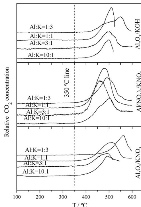
Fig. 3. Profiles of the catalysts prepared with Al<sub>2</sub>O<sub>3</sub>/KNO<sub>3</sub>, Al(NO<sub>3</sub>)<sub>3</sub>/KNO<sub>3</sub> and Al<sub>2</sub>O<sub>3</sub>/KOH precursor combinations after heat-treatment at 600 °C for 48 h.
