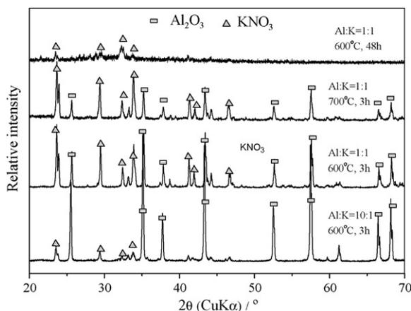
Fig. 4. XRD patterns of the catalysts prepared by  $\text{Al}(\text{NO}_3)_3/\text{KNO}_3$  at various conditions.
