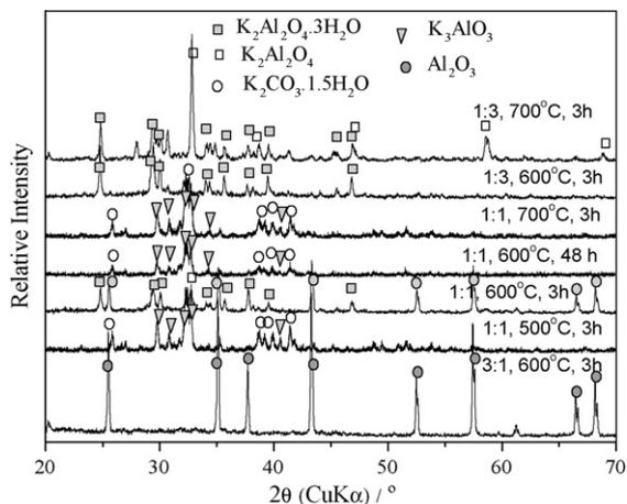
Fig. 5. XRD patterns of the catalysts prepared by  $\text{Al}_2\text{O}_3/\text{KOH}$  at various conditions.
