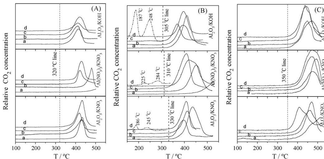
Fig. 2. TPR profiles of the catalysts prepared using various precursor combinations and calcination conditions of (A) 500 °C, 3 h, (B) 600 °C, 3 h and (C) 700 °C, 3 h at Al:K atomic molar ratios of (a) 10:1; (b) 3:1; (c) 1:1; (d) 1:3 (the dot lines in (B) are the blank test results of catalysts prepared with a Al:K molar ratio of 3:1).
