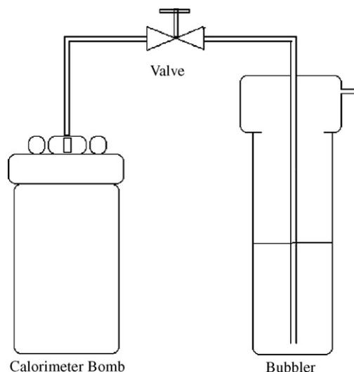
Fig. 1. System utilised for scrubbing the combustion gas from the calorimeter bomb.
