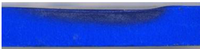
Fig. 10. Microscope image of toner sample after SPM probe analysis. Darker area indicates melted toner particles due to heat radiated from probe tip. Sample thickness is approximately 6 mm.
