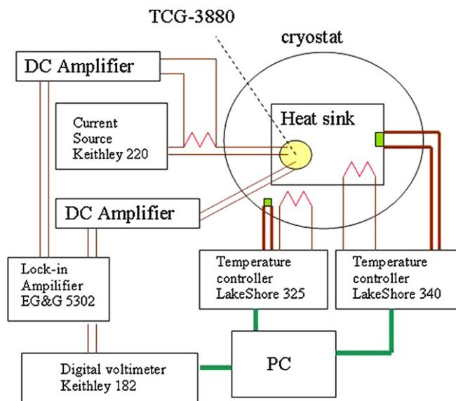
**Fig. 1.** Block diagram of the AC-calorimetry used for this experiment. The heater current is supplied by the current source and detected by the lock-in amplifier. The frequency of the excitation currents are variable from DC to  $150\ \text{Hz}$ .
