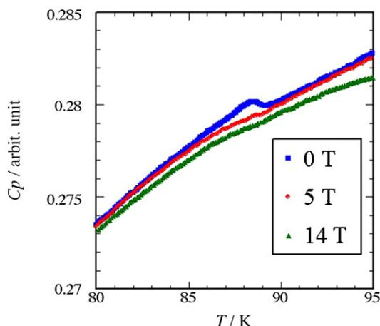
Fig. 3. Temperature dependence of the ac-heat capacity of  $\text{YBa}_2\text{Cu}_3\text{O}_{7-\delta}$  obtained under 0 T and with magnetic fields of 5 and 14 T.
