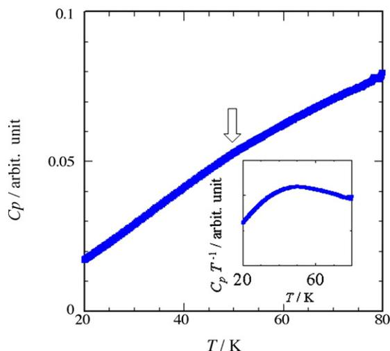
Fig. 4. Temperature dependence of the ac-heat capacity of organic charge transfer salt of  $(\text{DMe-DCNQI})_2\text{Li}$  which is known to show spin-Peierls transition at 51 K.
