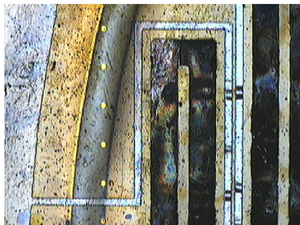
Fig. 14. Optical photograph of the thermal open circuit avoiding lateral heat loss. Few micro-posts in yellow (gold) are visible in the bottom of the trench. The width of the platinum wire crossing the trench is only of 30 \mu\text{m} . (For interpretation of the references to color in this figure legend, the reader is referred to the web version of the article.)
