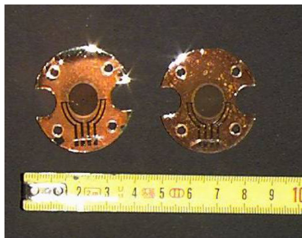
Fig. 12. Complete cell for liquid measurement. One contains the heater and the other the thermometer. A transparent thin spin coated polyimide film, less than 1 \mu\text{m} thick, electrically insulates the sensitive elements from the liquid sample.
