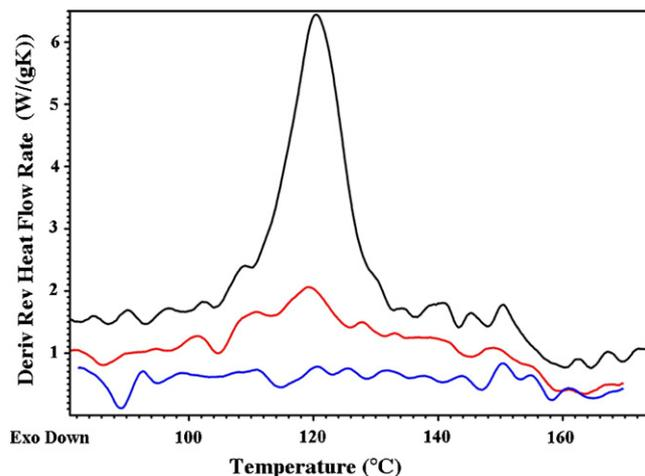
**Fig. 5.** The derivative of the heat flow rate for PMMA adsorbed on silica as a function of temperature for 10% (bottom), 30% (middle) and 70% (top) PMMA.
