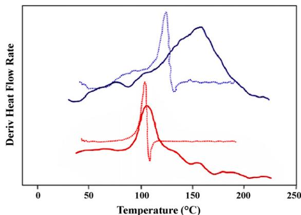
Fig. 7. Thermograms of PS (lower) and PMMA (upper) in bulk (dashed) and on silica (solid). The adsorbed amounts were 1.23 and 1.30 mg/m<sup>2</sup> for PS and PMMA, respectively.
