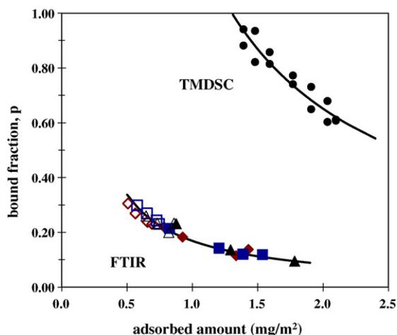
**Fig. 3.** Bound fractions of PMMA,  $p$ , from FTIR (carbonyls, lower) and TMDSC (upper).
