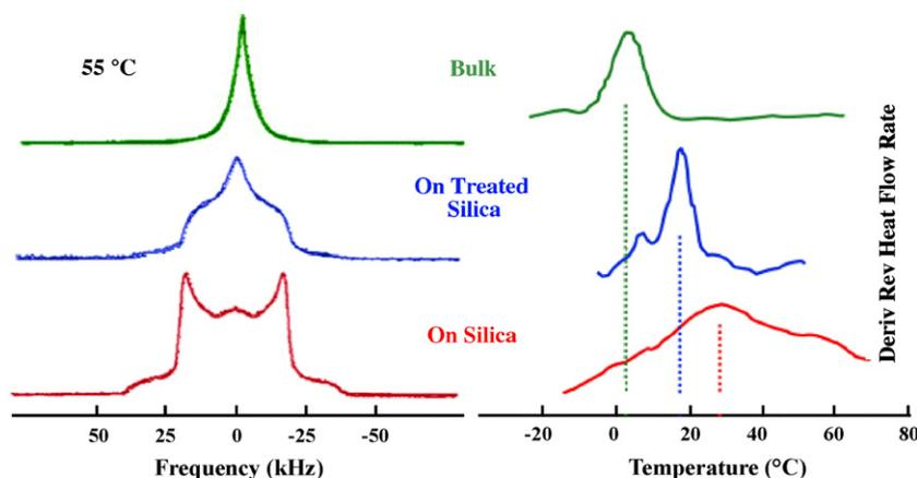
**Fig. 8.** Solid-state  $^2\text{H}$  NMR spectrum of PMA- $\text{d}_3$  at 55 °C (left) and derivative TMDSC thermograms of PMA (right) in bulk (upper), on treated silica (middle), and on native silica (lower).
