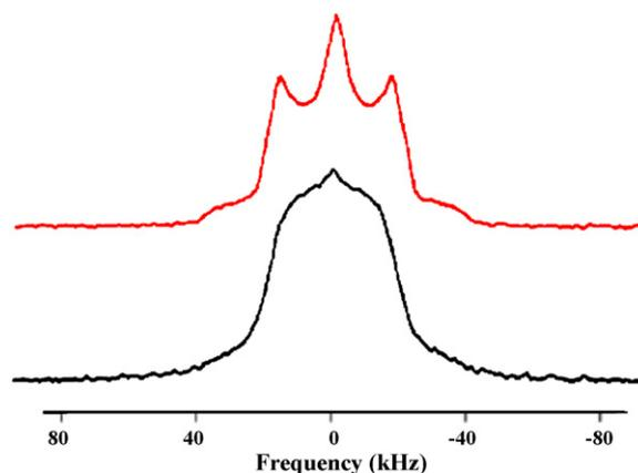
Fig. 6. Solid-state <sup>2</sup>H NMR spectra of PVAc-d<sub>3</sub> in bulk (lower) and at 0.36 mg/m<sup>2</sup> adsorbed on silica (upper) at 68.8 °C. The spectrum of the adsorbed polymer shows the presence of segments that were more mobile and those that are less mobile than those in the bulk polymer.
