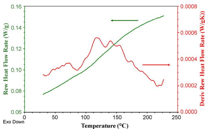
**Fig. 4.** DSC thermogram for adsorbed PMMA on silica ( $0.80\text{ mg/m}^2$ ) showing the heat flow rate and also the derivative of the heat flow rate.
