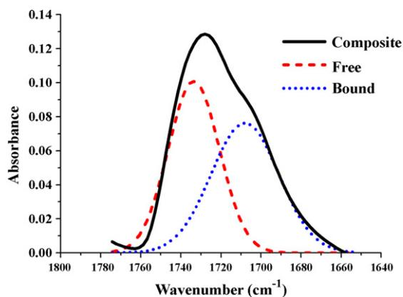
**Fig. 2.** FTIR spectrum of the carbonyl stretching region for PMMA adsorbed on Cab-O-Sil showing the component spectra due to free ( $1734\text{ cm}^{-1}$ ) and hydrogen-bonded ( $1708\text{ cm}^{-1}$ ) carbonyls.
