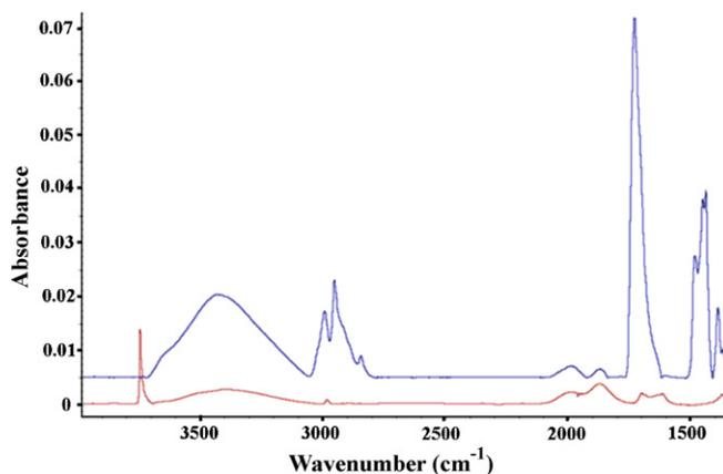
**Fig. 1.** FTIR spectrum of Cab-O-Sil (lower) and 0.6 mg/m<sup>2</sup> PMMA adsorbed on Cab-O-Sil (upper). The resonance at 3745 cm<sup>-1</sup> is from the free surface silanols on Cab-O-Sil.
