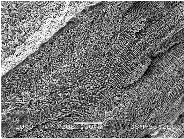
Fig. 3. SEM micrograph of the glass ceramics no. A3.
