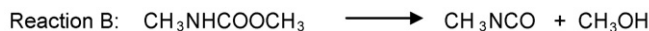
Scheme 2. Thermolysis reaction of N,N-dialkyl carbamates (reaction A) and mono-substituted carbamates (reaction B).
