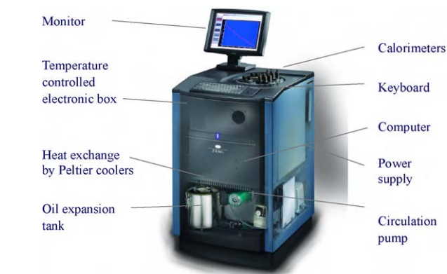
Fig. 1. Structure of thermal activity monitor III [13].
