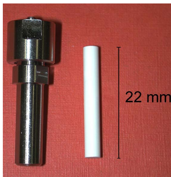
Fig. 2. Left: a stainless steel crucible developed for the DSC measurements of volatile samples; right: boron nitride liner which is inserted into the crucible to separate the sample and the main body of the crucible.
