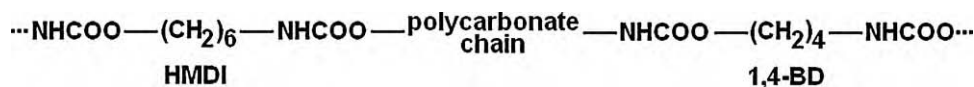
Fig. 1. The structure of polyurethane chains synthesized from polycarbonate diol, hexamethylene-diisocyanate (HMDI) and 1,4-butanediol (1,4-BD).
