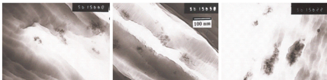
Fig. 1. TEM micrographs of PET/SiO 2 nanocomposites containing (a) 0.5 wt%, (b) 2 wt% and (c) 4 wt% SiO 2 .
