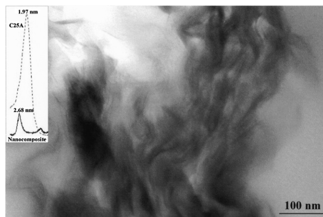
Fig. 1. Transmission electron micrograph showing the morphology of the poly(glc- alt -amh)/C25A nanocomposite with a Cloisite concentration of 3%. Inset shows the diffraction peak associated to the interlayer spacing observed in the C25A organo-modified clay (dashed line) and the nanocomposite sample (solid line).
