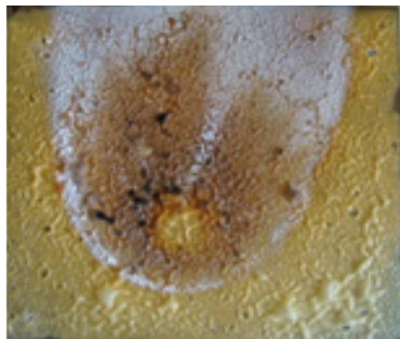
Fig. 4. Sample after the torch test.
