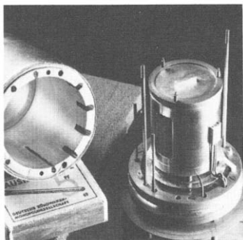
Fig. 5. Upper part of adiabatic shield is put aside, inner vessel with graphite container for the probe can be seen
