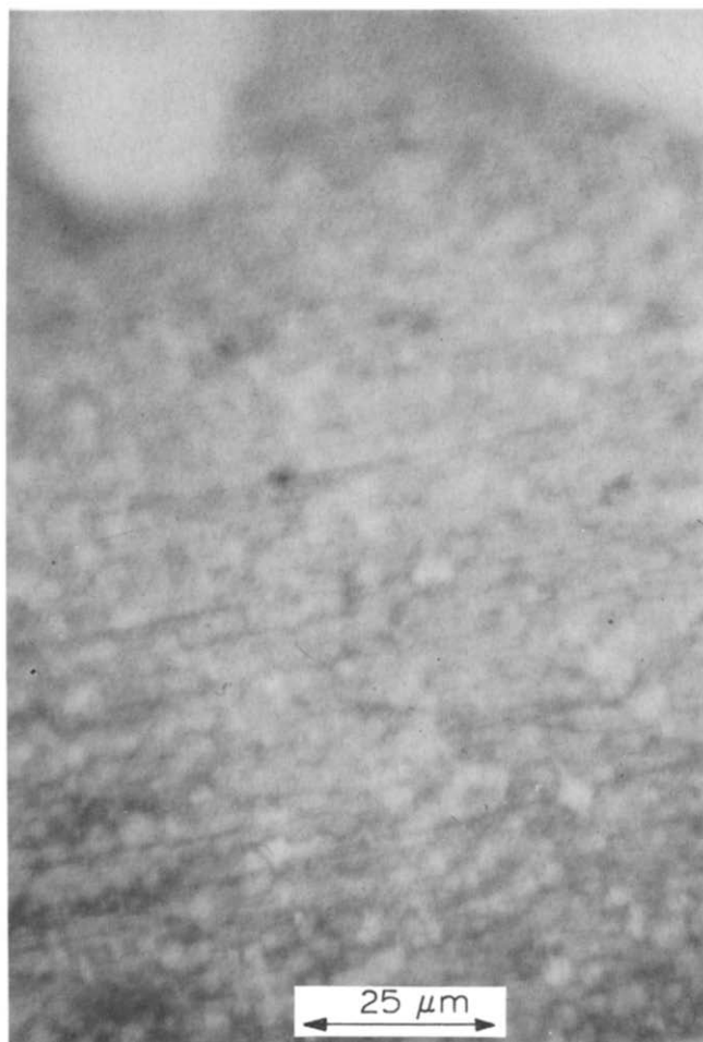
Fig. 1. Mesophase spherules in naphthalene heat-treated to 538^\circ\text{C} for 5 h.
