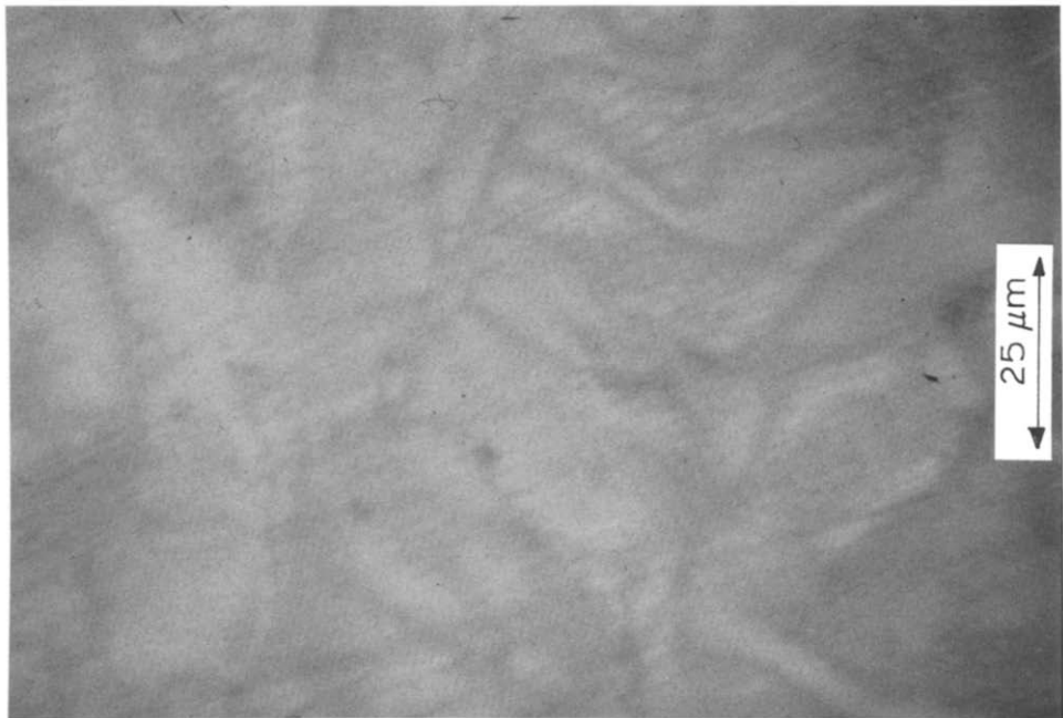
Fig. 9. Mosaic formation in phenanthrene heat-treated to 550°C for 5 h.
