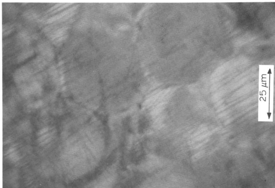
Fig. 5. Mesophase development in anthracene heat-treated to 480°C for 2 h.
