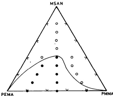
Fig. 2. Phase diagram of MSAN/PMMA/PEMA blends.
