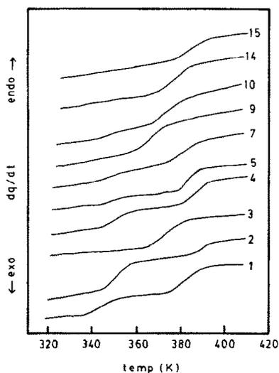
Fig. 1. DSC curves of several MSAN/PMMA/PEMA ternary blends; each number refers to the sample number in Table 1.
