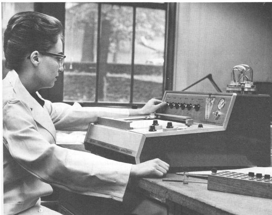
Fig. 5. Judy Clark of the Polychemicals Department at Du Pont using an early model of the Du Pont 900 DTA.
