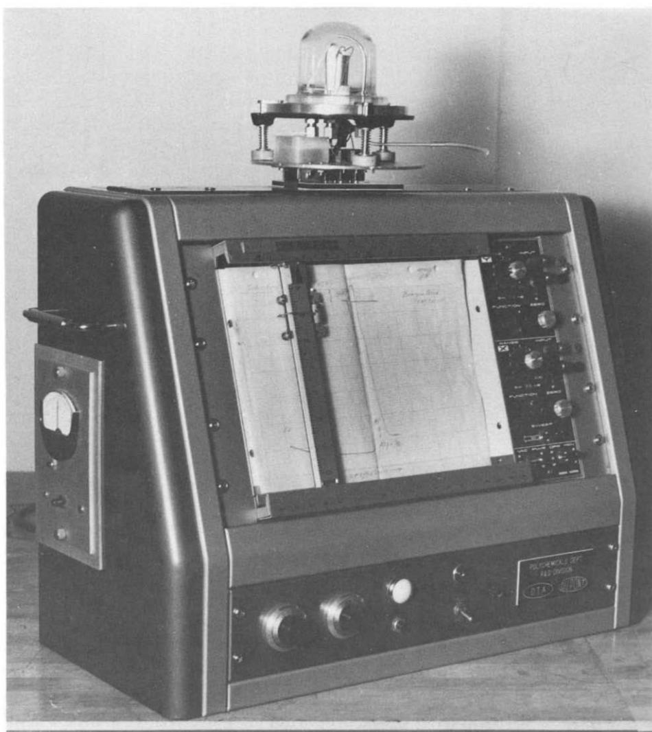
Fig. 2. A more compact early model of a Differential Thermal Analyzer in 1962.
