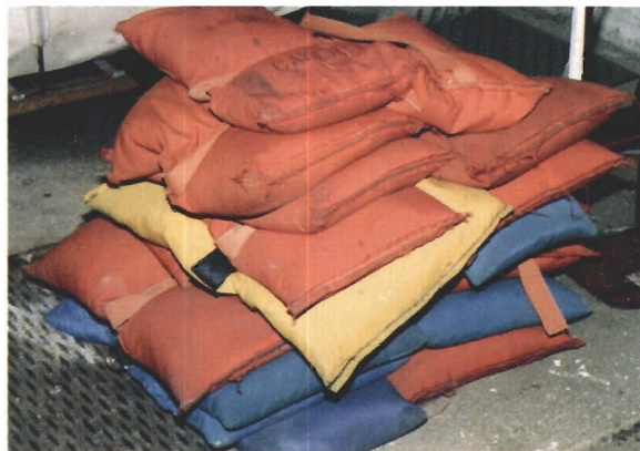
Sandbags are handy stabilizers for lighting stands and gear.
