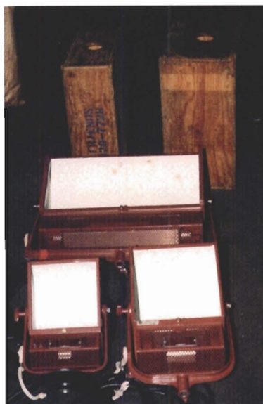
Three sizes of spotlights plus two all-purpose plywood "apple" boxes.
