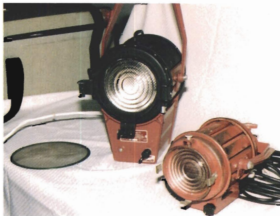
These spotlights with fresnel-type lenses can be adjusted between flood and spot via the black knob below the lens.
