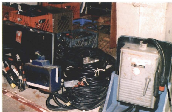
"Tie-in" equipment adds big bucks to your lighting truck income. From left to right: stage plugs, four-way cables and tie-in box.
