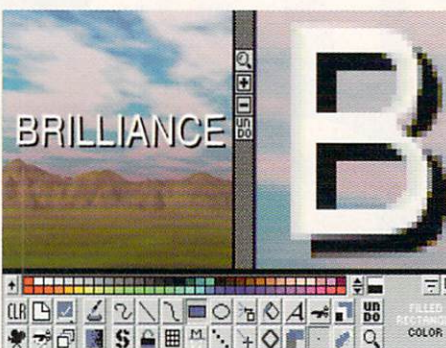
HAM8 display showing magnification and antialiasing.
