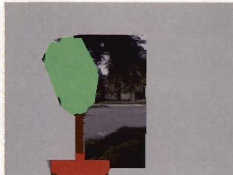
Backflat: This is what your final rendering of the Backdrop, Wall and Plant may look like. The beauty, however, is that this scene is composed of only three polygons. Using a photo of a wall, you can add detail to the gray surface. Some careful cropping of the Plant object can give realistic shape to the leaves. Copyright 1994 Avekta Productions Inc.
