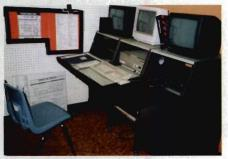
This networked 3D workstation has a A2500 with 68040, PAR, TBC IV and an external 640 MB drive.
