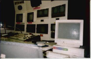
The production control room includes an A4000 with a Super Gen SX Genlock. The A4000 is the end of a 23 station network and the conduit for all work to go to broadcast.
