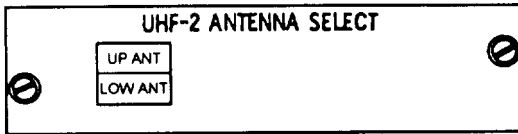
Figure 1-9.-UHF-2 antenna select panel.
