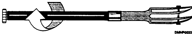
Figure 2-33. —A railroad pen with rotating handle.
