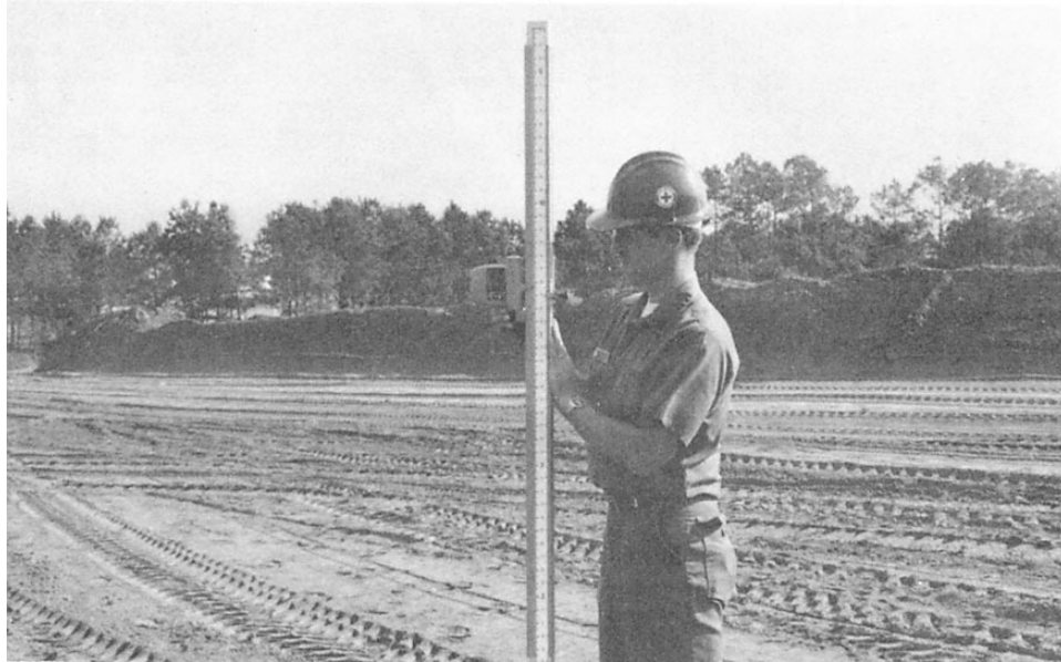
Figure 12-7.—Laser-level rod equipped with a laser detector.
