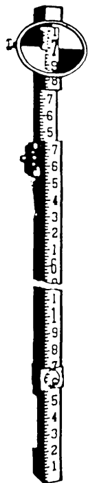
Figure 15-43.—Philadelphia level rod with target.
