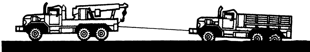
Figure 5-6.-Simple winch operation (direct pull).
