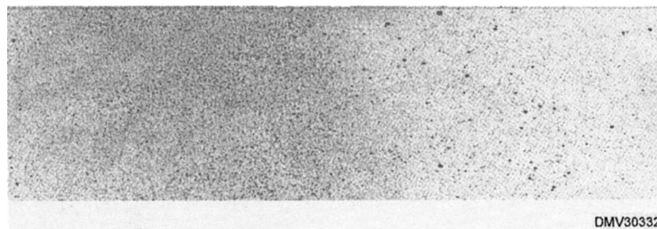
Figure 6-27. —Splatter created by air pressure in excess of 25-30 PSI.
