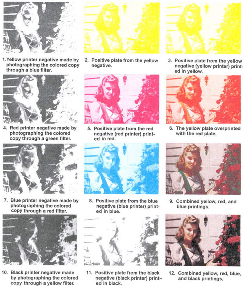
Figure 2-27. —Separation negatives, progressive proofs, and finished four-color image.
