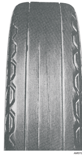
Figure 7-27.—Rapid tread wear caused by overinflation.
