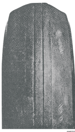
Figure 7-26.—Rapid tread wear caused by underinflation.
