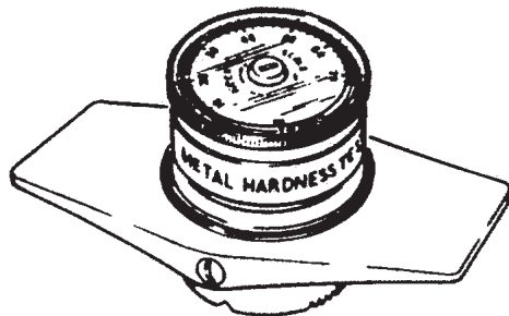
THE ERNST PORTABLE HARDNESS TESTER HAS A DIAMOND-TIPPED PENETRATOR AND READS IN ROCKWELL OR BRINELL SCALES.
