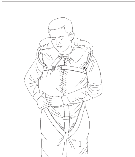
C. BOTH STRAPS PULLED BETWEEN LEGS, ONE FASTENED TO D RING ON LEFT SIDE, OTHER BEING FASTENED.
