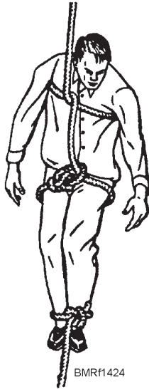
Figure 14-24.—Emergency rescue line.
