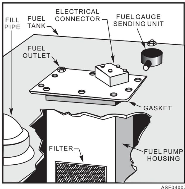
Figure 4-7.—Tank unit type of electric pump.
