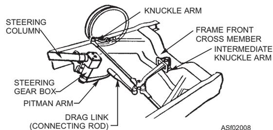
Figure 2-8.—Steering assembly.
