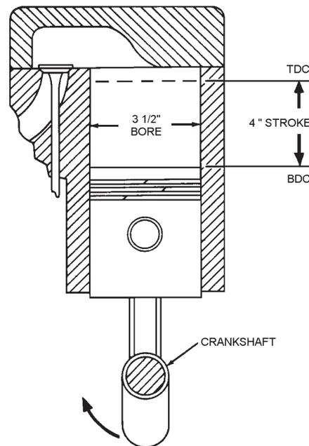
Figure 3-12.—Bore and stroke of an engine cylinder.
