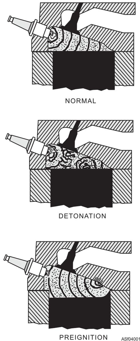
Figure 4-1.—Combustion process.
