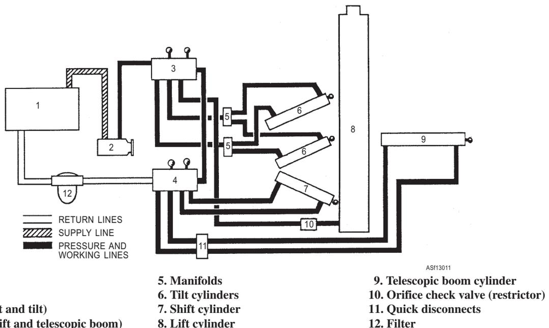
Figure 13-11.—Schematic of a typical forklift hydraulic system.
