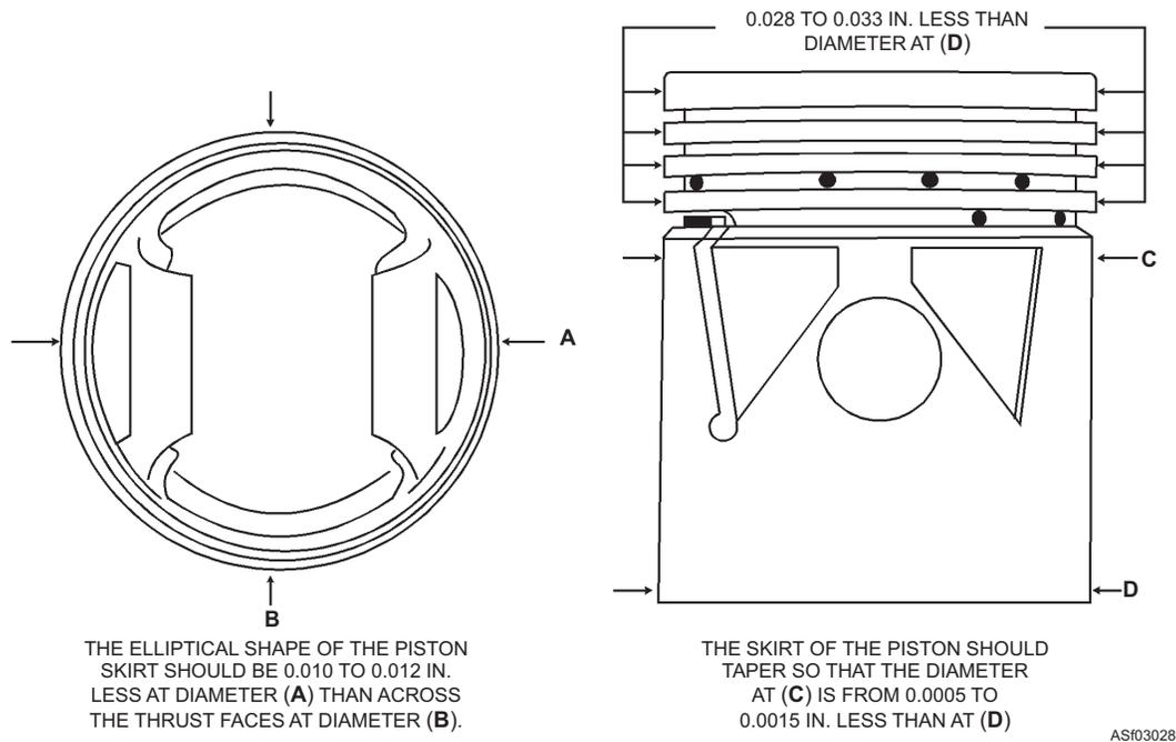
Figure 3-28.—Cam-ground piston.
