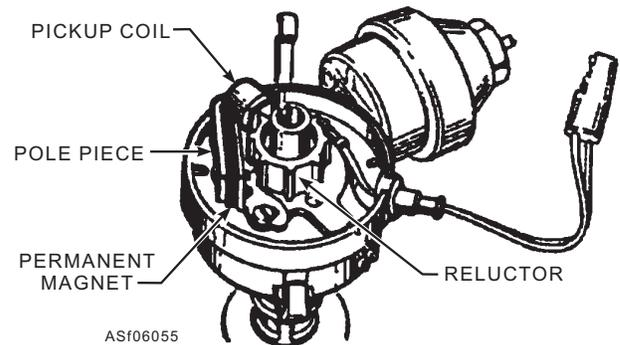
Figure 6-55.—Distributor used with transistorized ignition system.
