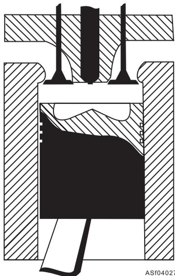
Figure 4-27.—Diesel engine open combustion chamber.
