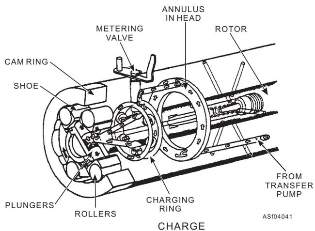
Figure 4-41.—Rotor in charging position with the rollers between the cam lobes (DC pump).
