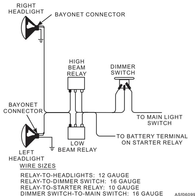
Figure 6-99.—Light relay wiring diagram.
