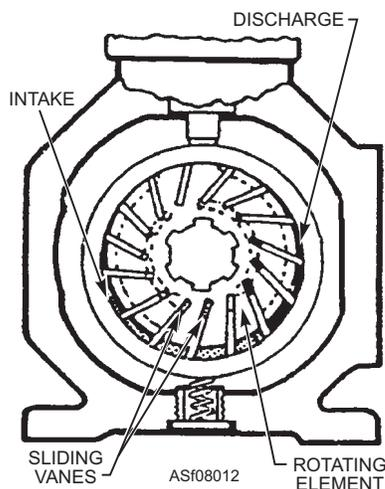
Figure 8-12.—Vane pump.
