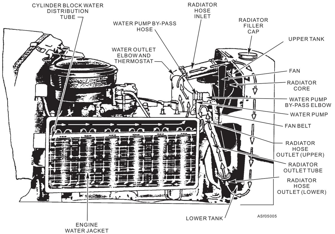
Figure 5-2.—Liquid-cooling system.
