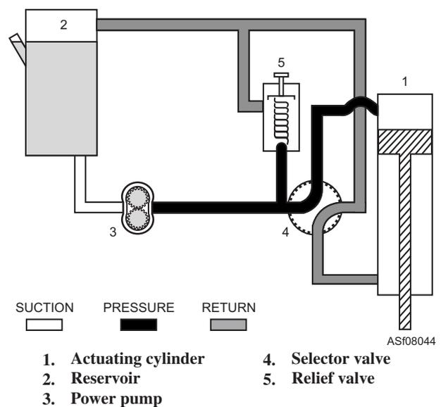
Figure 8-44.—Hydraulic system with a relief valve incorporated.
