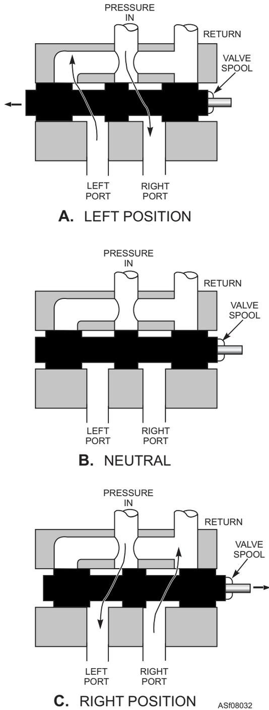
Figure 8-32.—Spool directional valve. ASf08032
