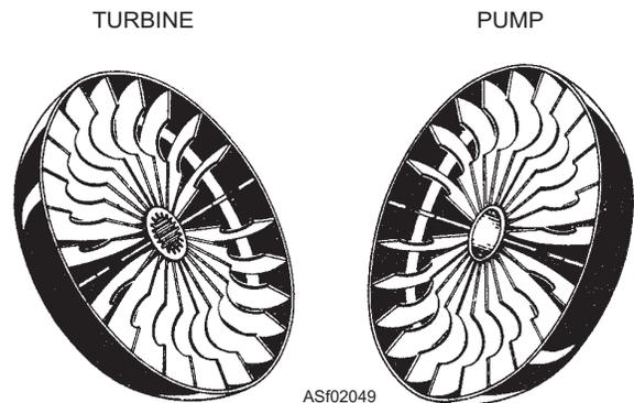
Figure 2-49.—Fluid coupling pump and turbine.
