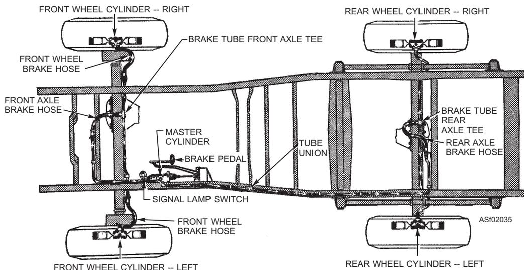
Figure 2-35.—Typical hydraulic brake system.
