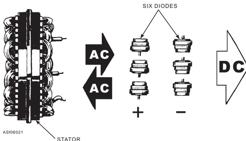
Figure 6-21.—Function of the alternator diode.
