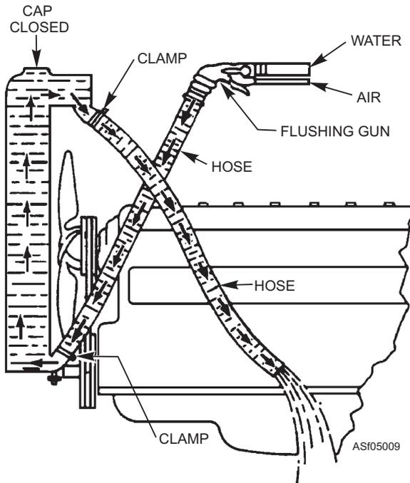
Figure 5-9.—Reverse flushing of radiator.
