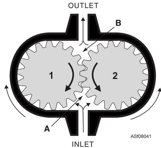
Figure 8-41.—Gear-type motor.
