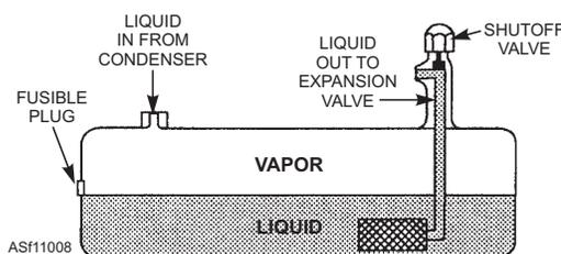
Figure 11-8.—Refrigerant receiver.
