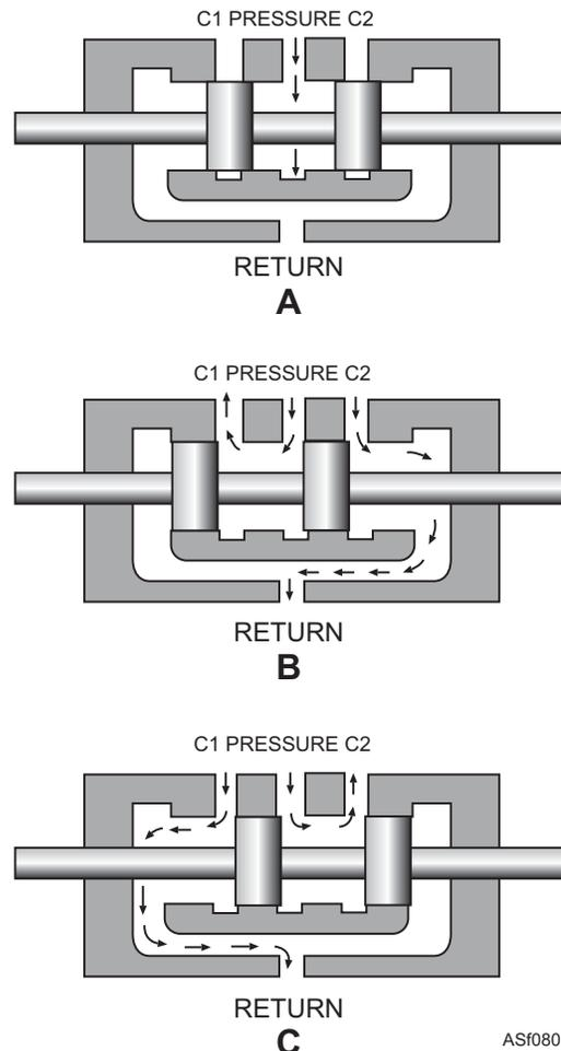
Figure 8-33.—Closed-center directional control valve. ASf08033
