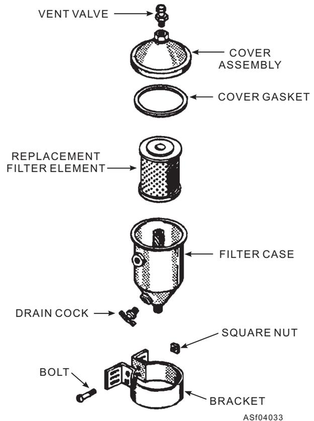
Figure 4-33.—Fuel filter assembly with replaceable element.
