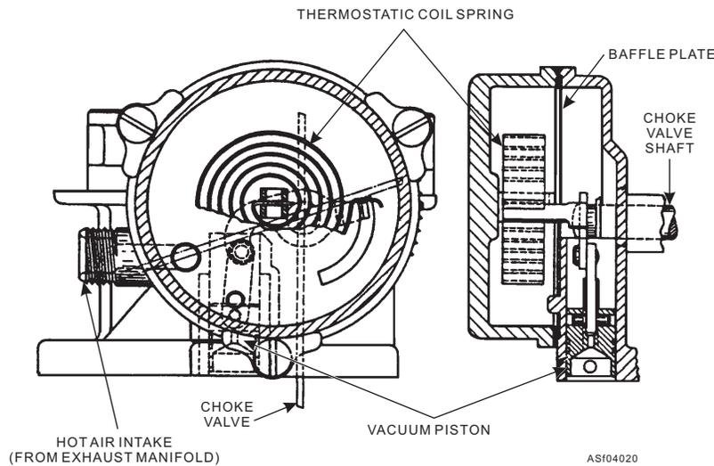
Figure 4-20.—Automatic choke.
