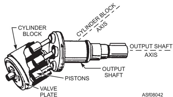
Figure 8-42.—Piston-type motor.
