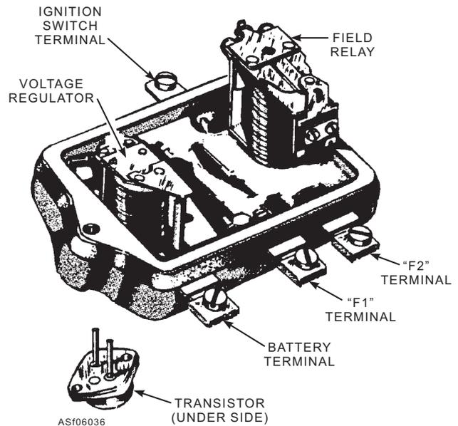
Figure 6-36.—Semitransistorized regulator.
