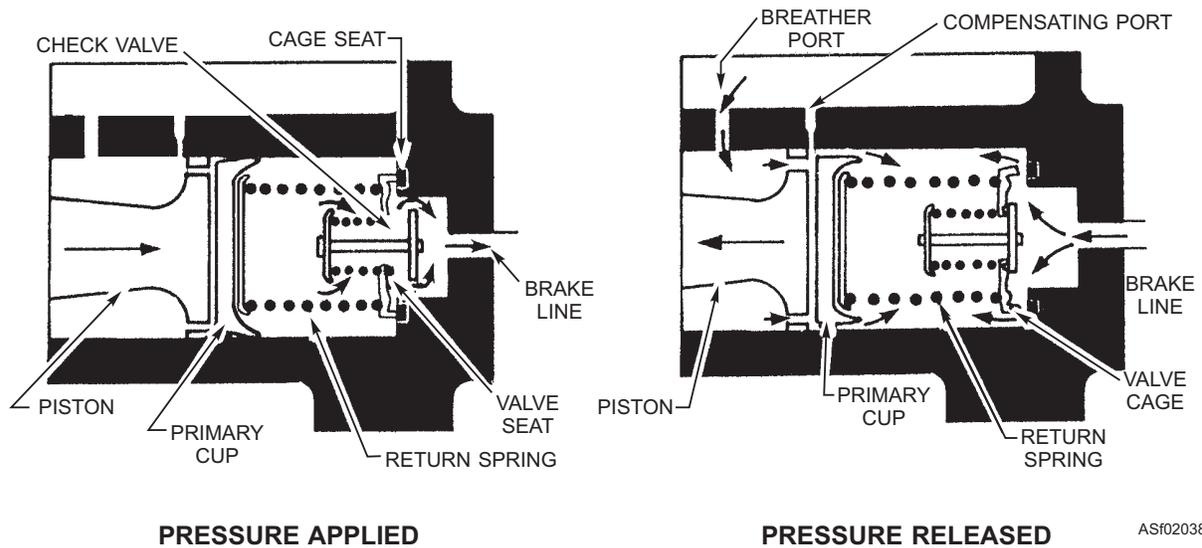
Figure 2-38.—Hydraulic brake master cylinder—operation of two-way valve.
