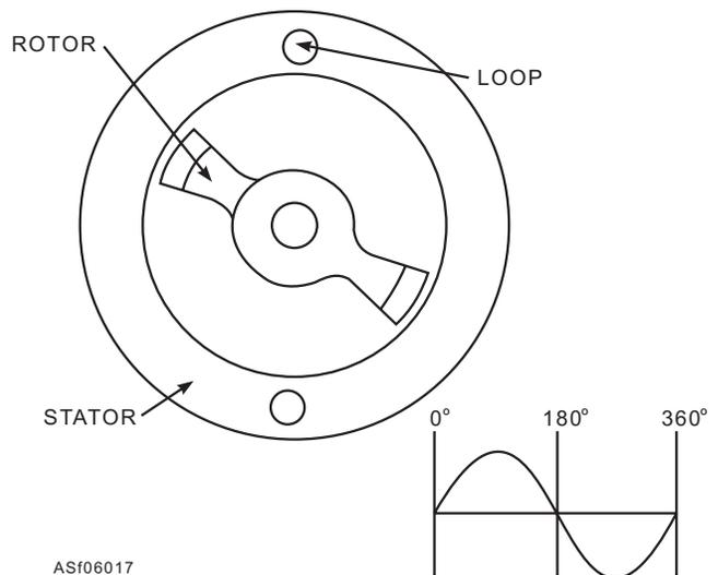
Figure 6-17.—A simple alternator.
