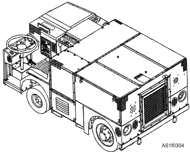
Figure 1-6.—A/S37A-3 shipboard mobile electric power plant.
