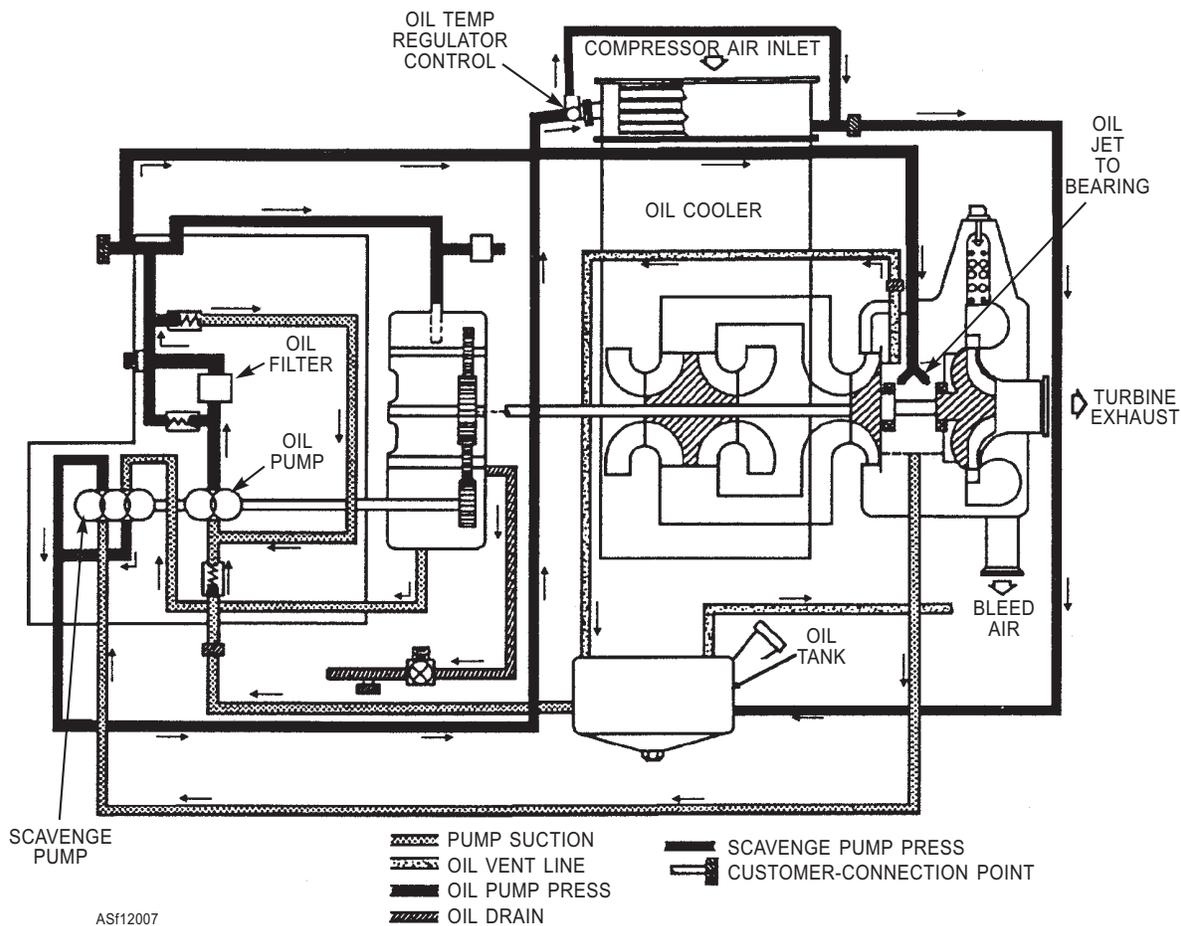
Figure 12-7.—Lubrication system.
