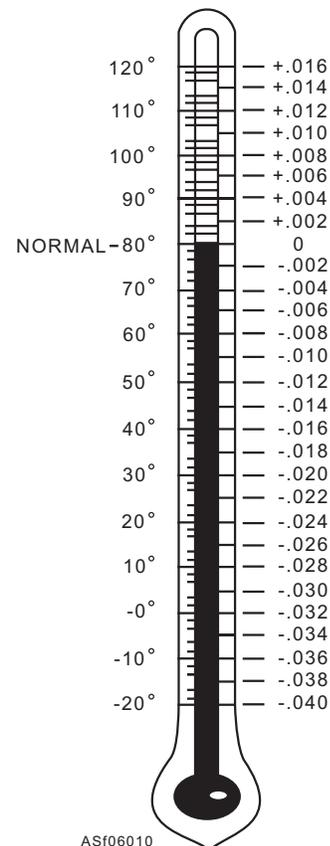
**Figure 6-10.—Specific gravity temperature correction chart.**
