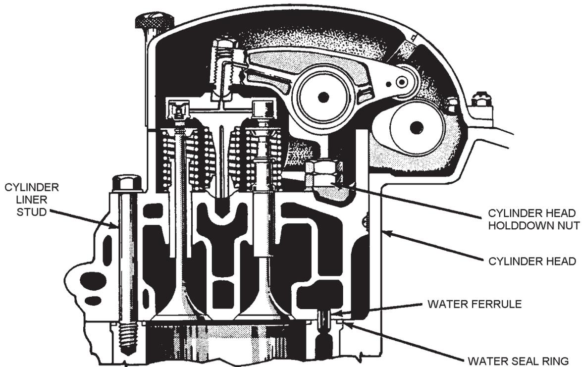
Figure 3-22.—Cylinder head for overhead valve engine.
