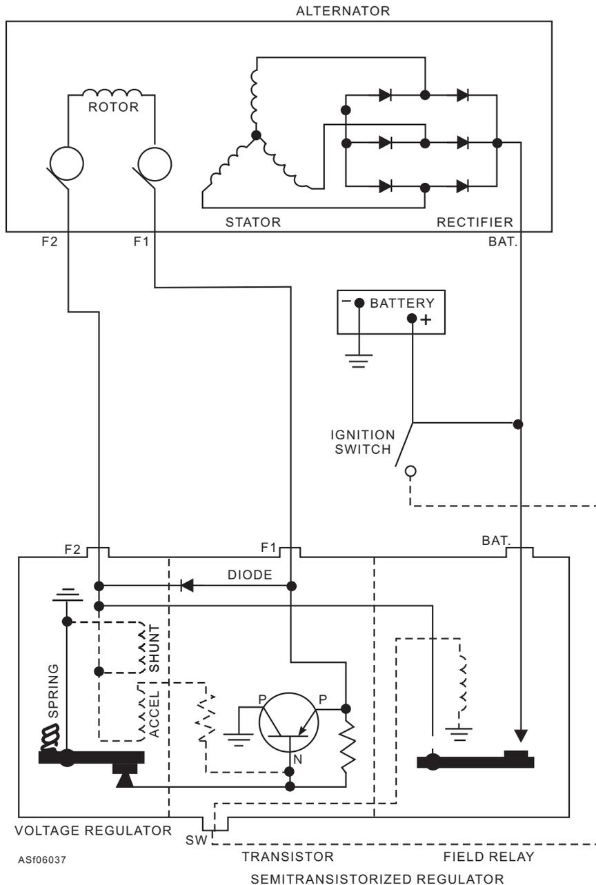
Figure 6-37.—Ac charging circuit using a semitransistorized regulator.
