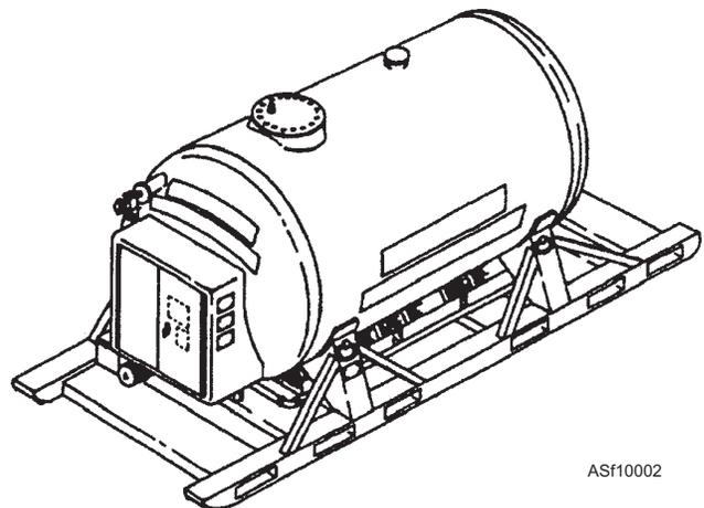
Figure 10-2.—2,000 gallon capacity liquid oxygen storage tank. ASF10002
