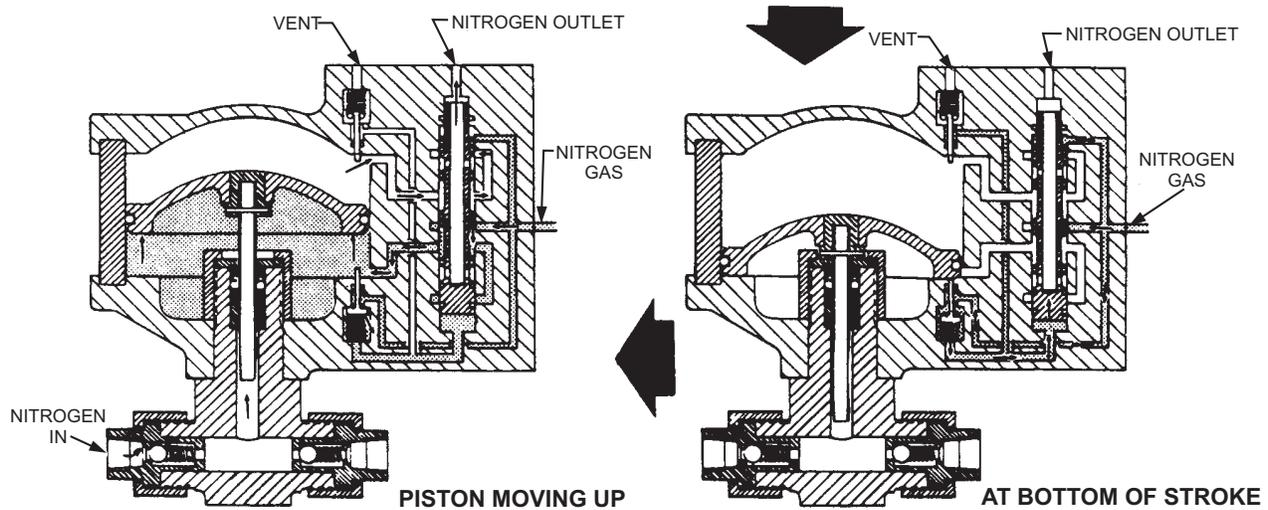
With control valve in RETURN position, supply nitrogen pressure acts on lower side of piston and moves it upward. This pushes the piston assembly up, sucking gas in thru inlet check valve. Nitrogen from upper side of piston is exhausted thru control valve spool.
