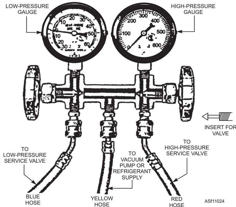
Figure 11-24.—Internal view of refrigerant manifold test set.
