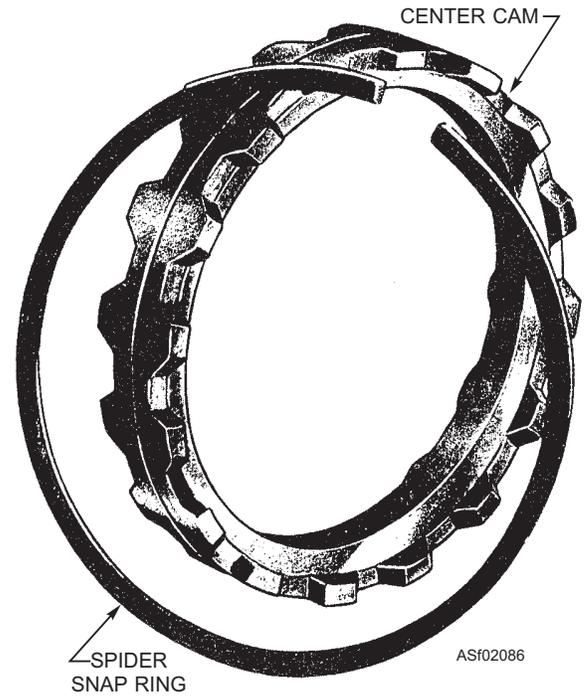
Figure 2-86.—Construction of center cam.
