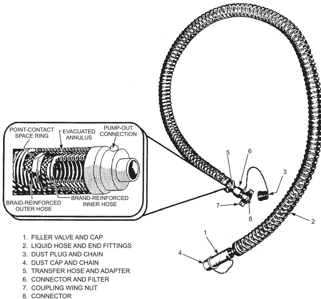
Figure 10-3.—Corrugated flexible metal hose.
