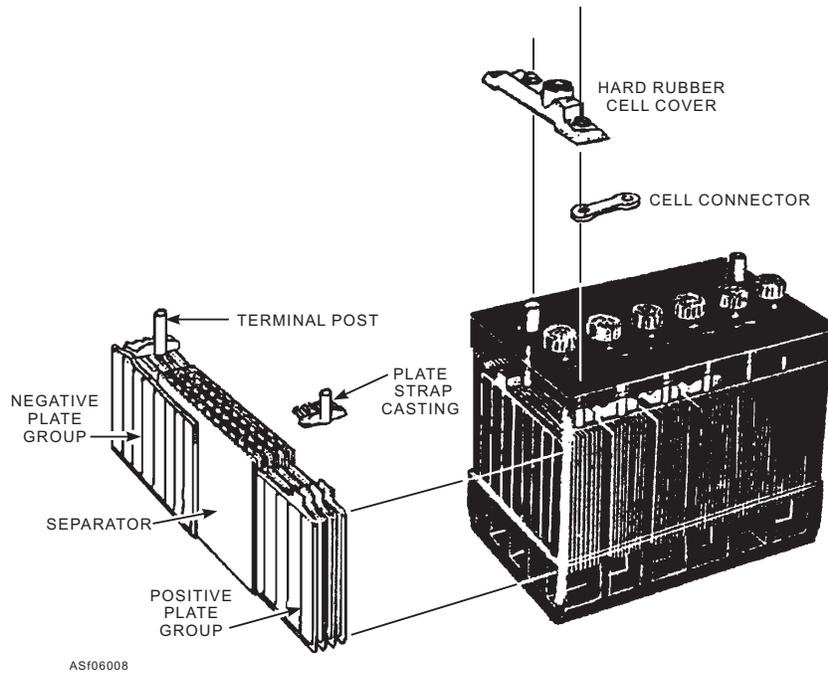
Figure 6-8.—Battery construction.
