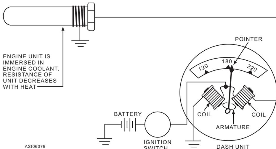
**Figure 6-79.—Electrical temperature gauge.**
