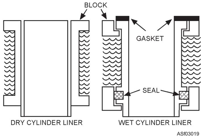
Figure 3-19.—Cylinder liner application.
