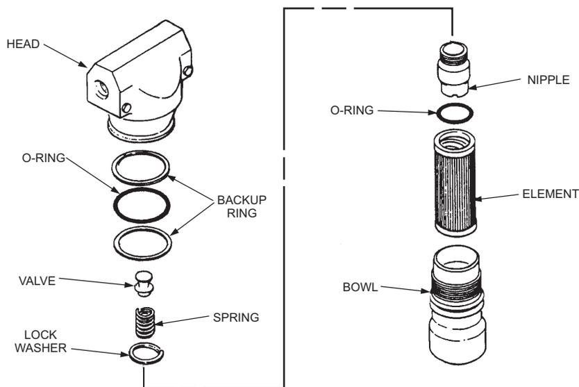
Figure 9-10.—Filter assembly.
