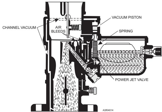
Figure 4-14.—Power jet full load circuit.
