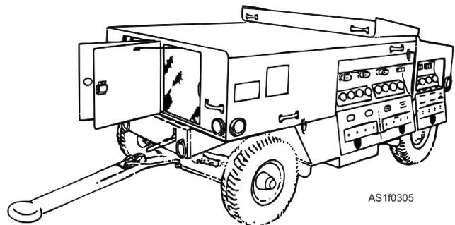
Figure 1-7.—DA-675/MSM dummy load electric unit.
