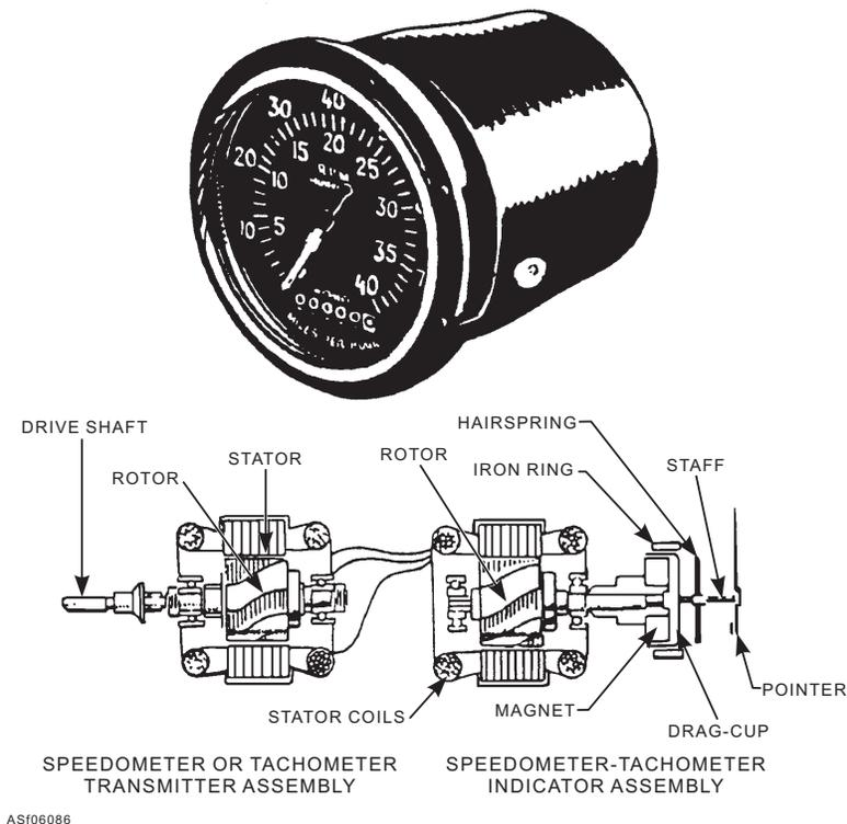
Figure 6-86.—Electrical speedometer-tachometer.
