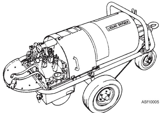
Figure 10-5.—TMU-70/M low-loss, closed-loop, liquid oxygen servicing trailer.
