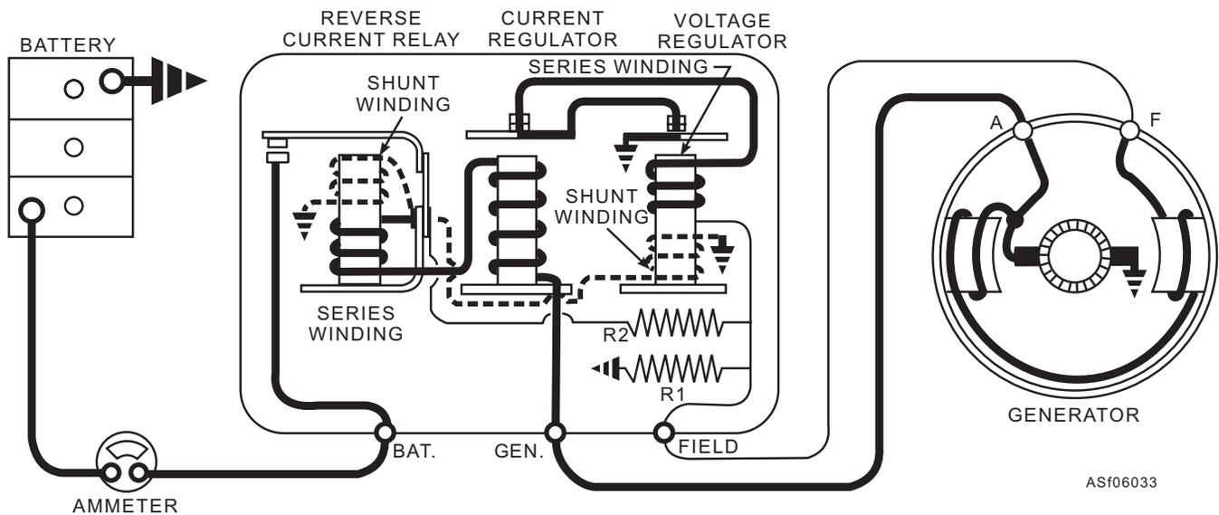
Figure 6-33.—Dc charging circuit with a vibrating-contact regulator.
