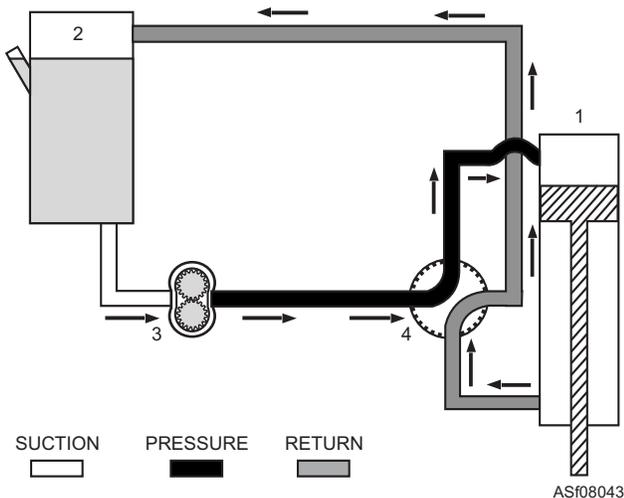
Figure 8-43.—Simple hydraulic system.
