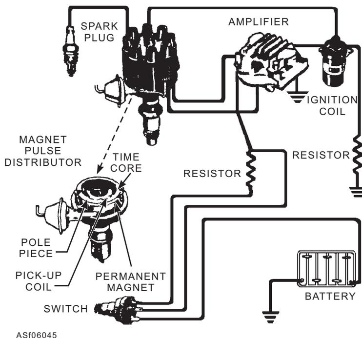
Figure 6-45.—Transistor controlled magnetic pulse battery ignition system.
