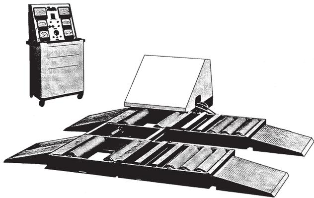
Figure 3-10.—Chassis dynamometer.
