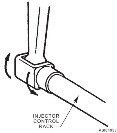
Figure 4-53.—Checking rotating movement of injector control rack.
