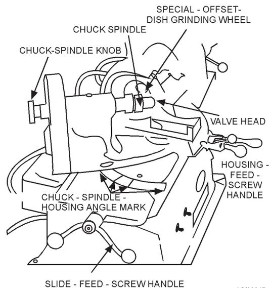
Figure 3-47.—Valve refacing machine.
