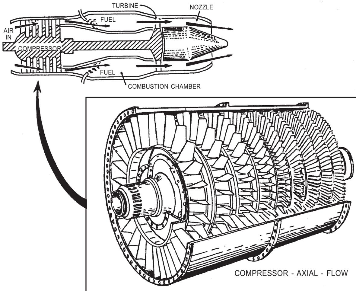
Figure 12-2.—Axial-flow type engine.
