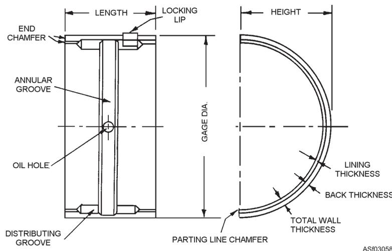
Figure 3-58.—Typical sleeve-type bearing half.
