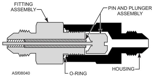
Figure 8-40.—Pressure gauge snubber.
