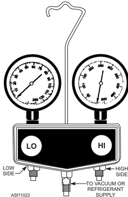
Figure 11-23.—Refrigerant manifold test set.
