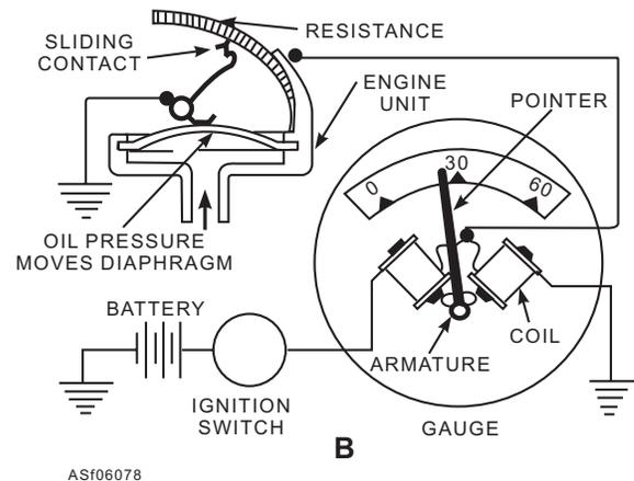
Figure 6-78.—(A) Oil pressure sending unit; (B) Schematic diagram of balancing coil oil pressure indicating system.
