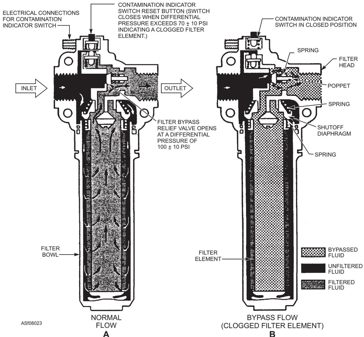
Figure 8-23.—Full flow bypass, electrical indicating hydraulic filter.
