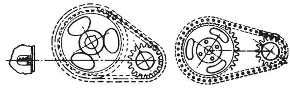
Figure 3-57.—Methods of valve timing with chain drive.
