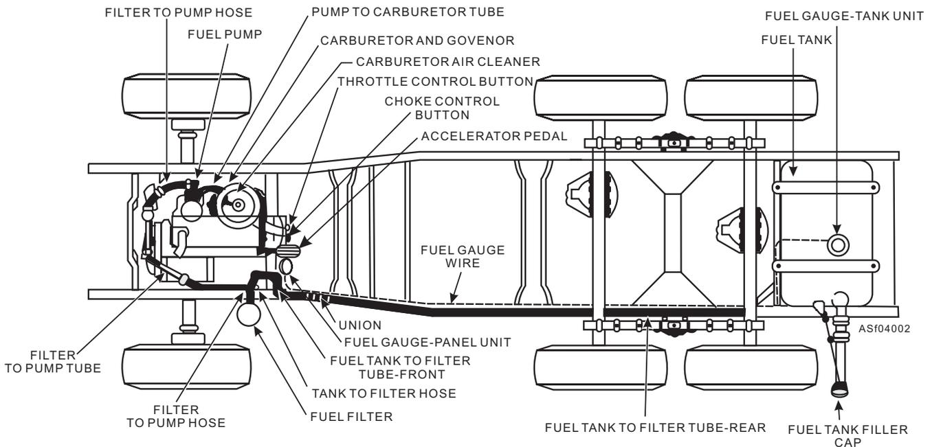
Figure 4-2.—Typical fuel system for a gasoline engine.
