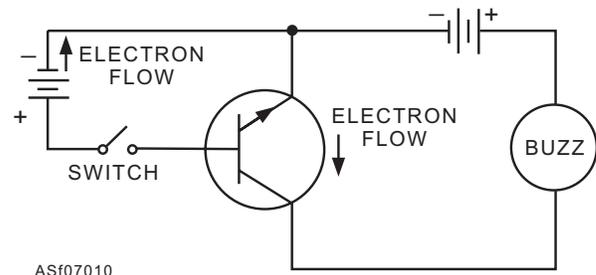
Figure 7-10.—Simple circuit using a transistor as a switch.
