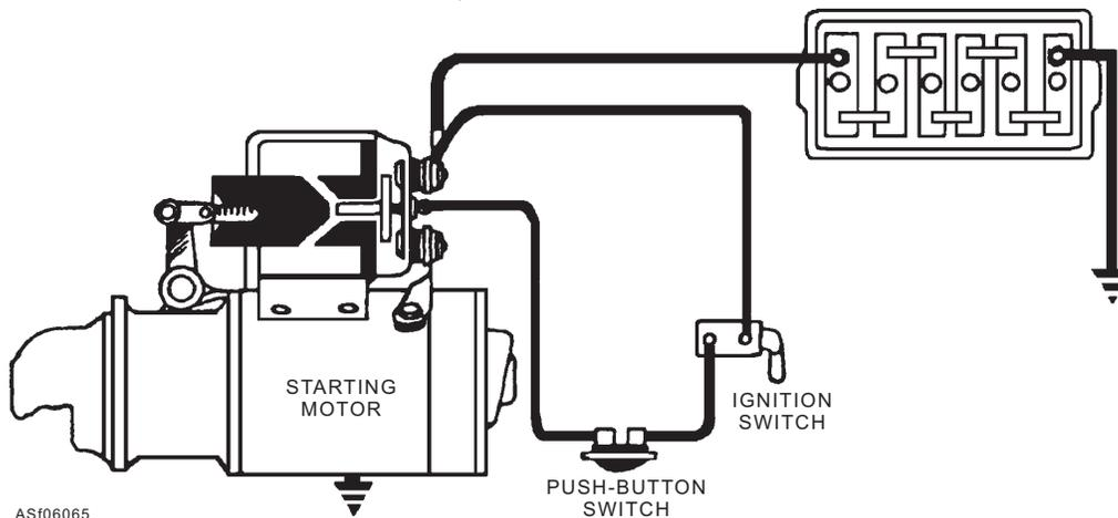
Figure 6-65.—Electric starting system.
