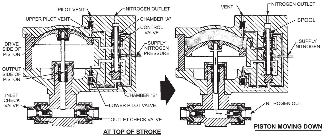
With piston in upper position, upper pilot valve is open. This exhausts chamber B. Supply nitrogen pressure in chamber A then moves control valve to DRIVE position.
