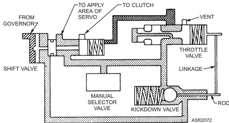
Figure 2-72.—Functional shift valve controls.
