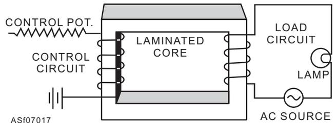
Figure 7-17.—A basic magnetic amplifier.
