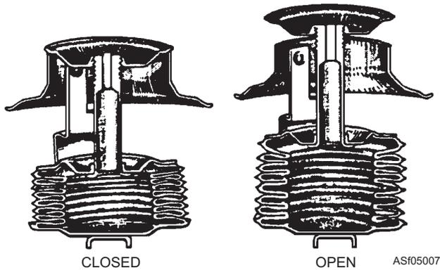
Figure 5-7.—Bellows thermostat.
