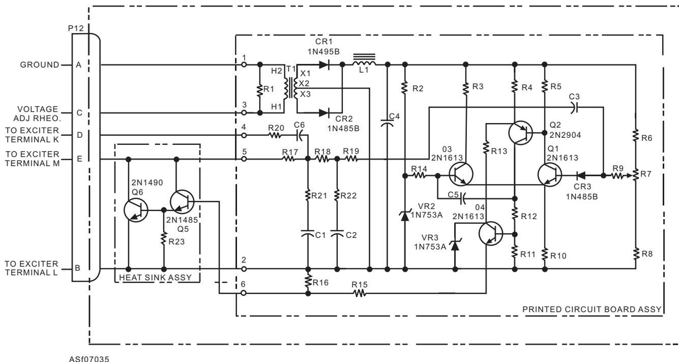
Figure 7-35.—An ac voltage regulator (VR2) simplified schematic.
