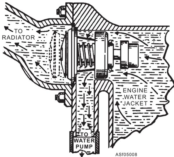
Figure 5-8.—Pellet thermostat.
