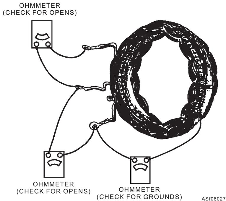
Figure 6-27.—Testing the stator for opens and grounds.
