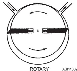
Figure 11-2.—Compressor types.
