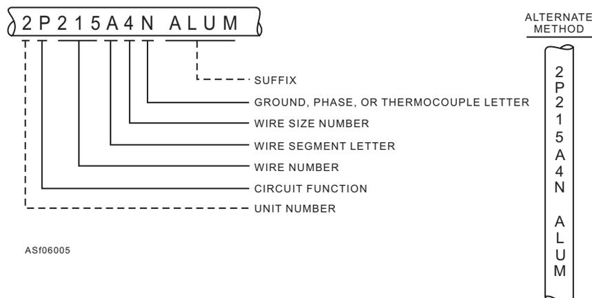
Figure 6-5.—Alphanumeric wire identification code.
