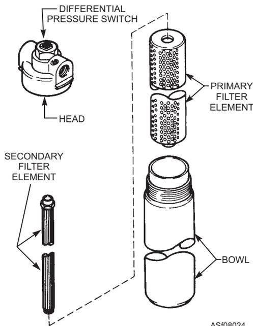
Figure 8-24.—High-pressure filter.
