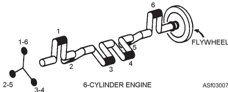
Figure 3-7.—Crankshaft for a 6-cylinder engine.
