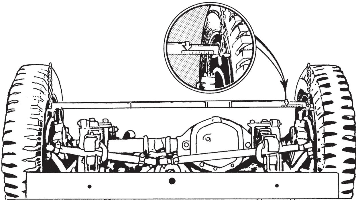
Figure 2-16.—Measuring pole.
