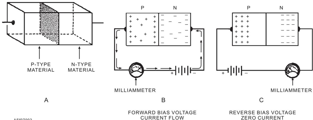
**Figure 7-2.—Junction diode.**
