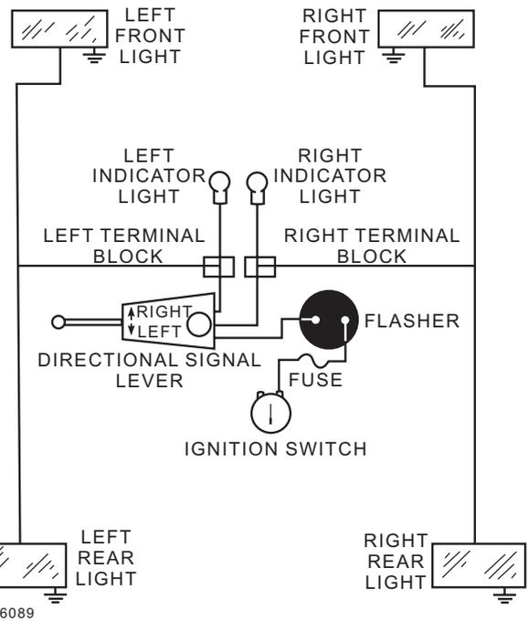
Figure 6-89.—Pictorial diagram of a directional signal system.
