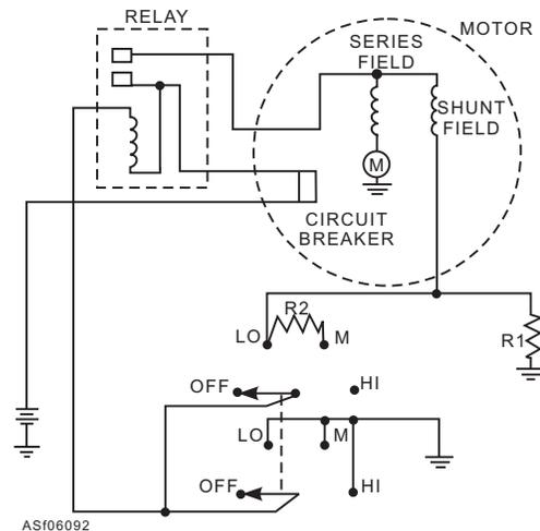
Figure 6-92.—Schematic diagram of a three-speed windshield wiper.
