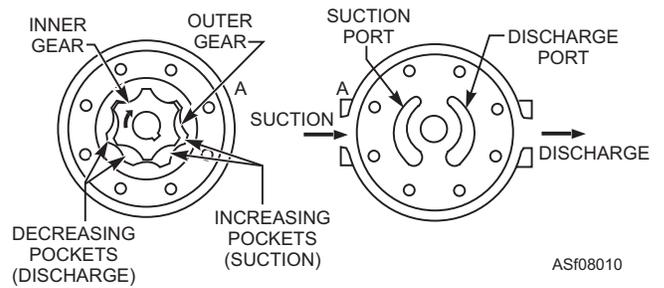
Figure 8-10.—Internal gear pump.
