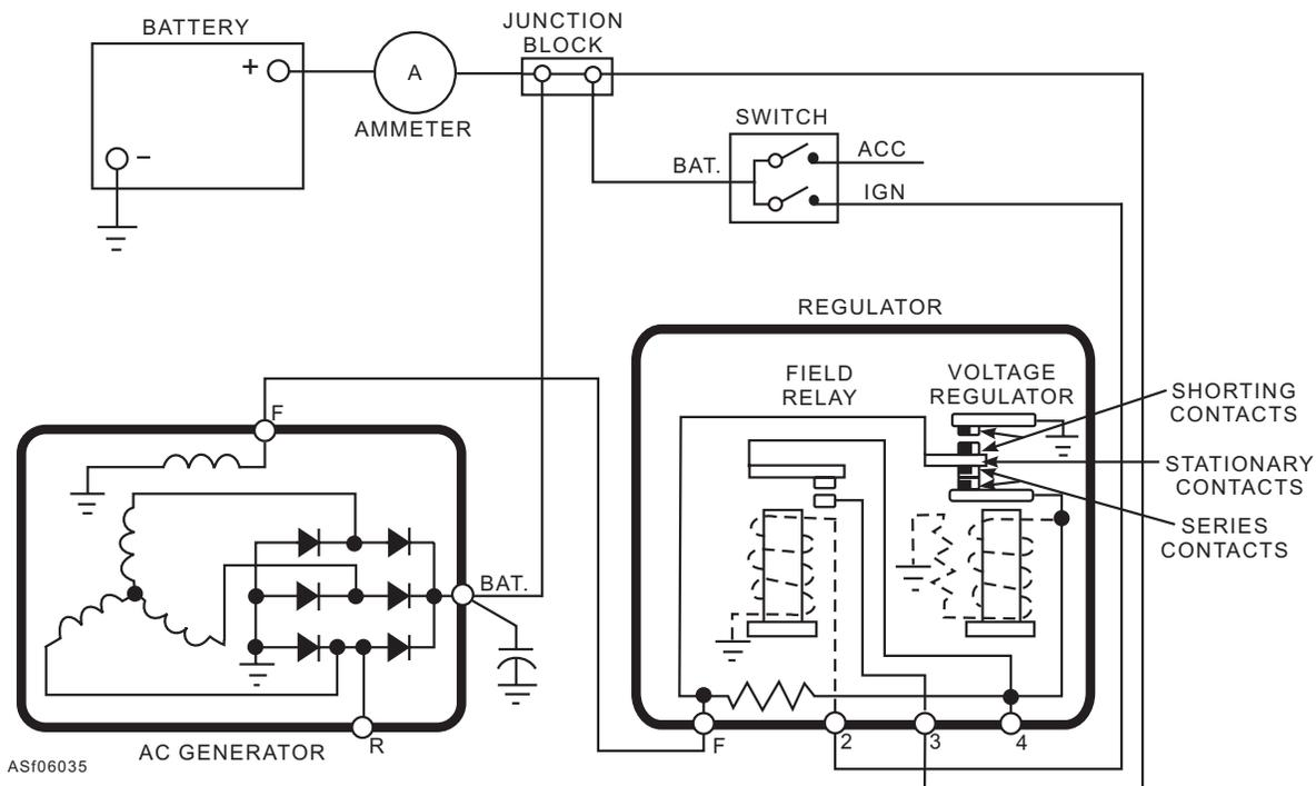
Figure 6-35.—Ac charging circuit using a vibrating-contact regulator.
