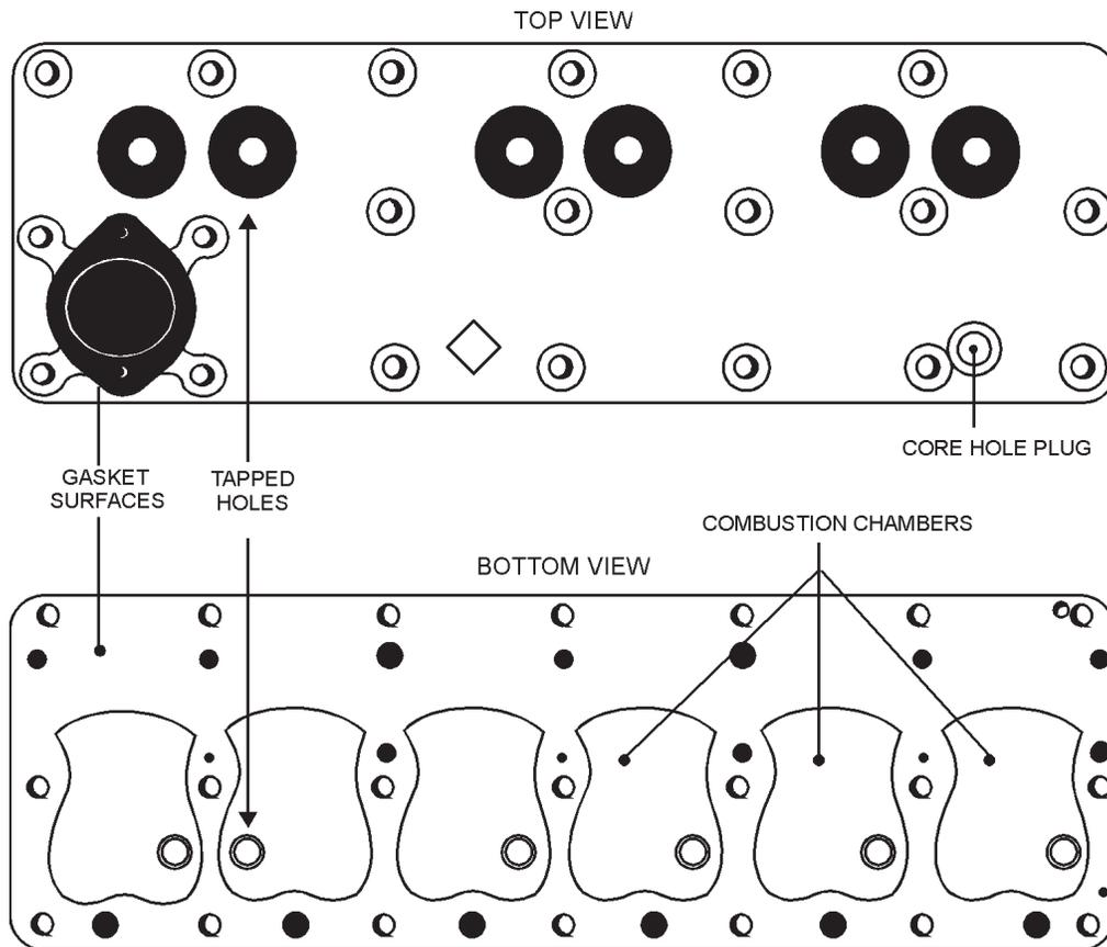
Figure 3-21.—Cylinder head for L-head engine.
